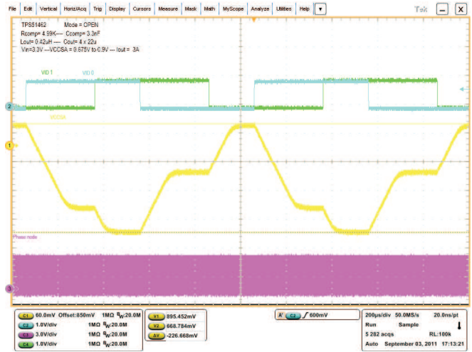
Figure 15. Mode=8, I OUT = 3 A, VID Transitions
