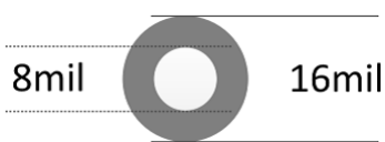
Figure 11-7. Recommended Minimum Via Sizing
