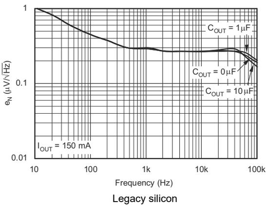
Figure 5-27. Noise Spectral Density  $C_{NR} = 0\mu\text{F}$
