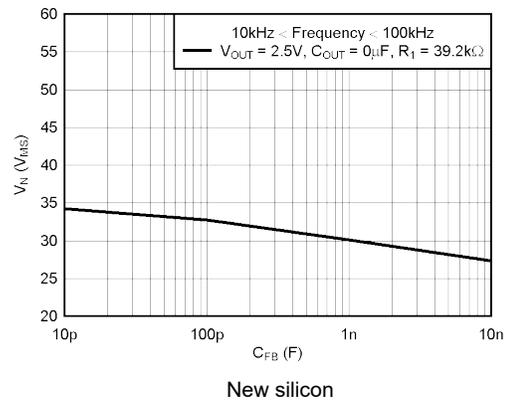
Figure 5-48. TPS73101 RMS Noise Voltage vs  $C_{FB}$
