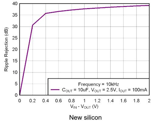
Figure 5-26. PSRR (Ripple Rejection) vs  $(V_{IN} - V_{OUT})$
