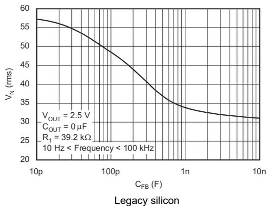
Figure 5-47. TPS73101 RMS Noise Voltage vs  $C_{FB}$
