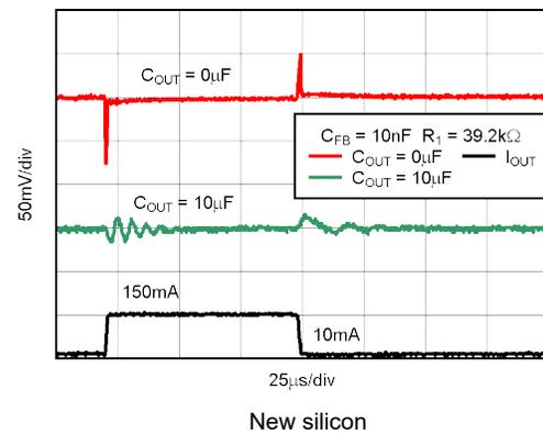
Figure 5-52. TPS73101 Load Transient, Adjustable Version
