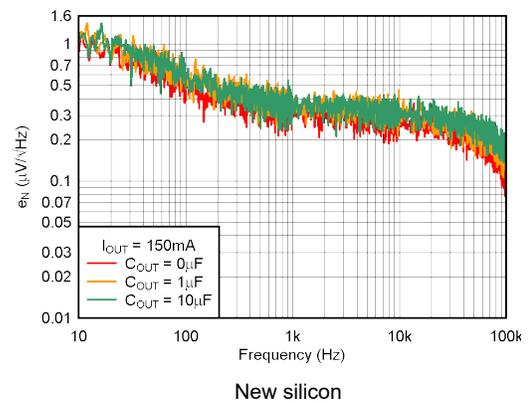
Figure 5-28. Noise Spectral Density  $C_{NR} = 0\mu\text{F}$
