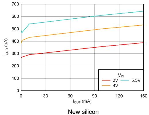
Figure 5-12. Ground Pin Current vs Output Current
