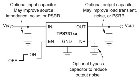
Figure 7-1. Typical Application Circuit for Fixed-Voltage Versions
