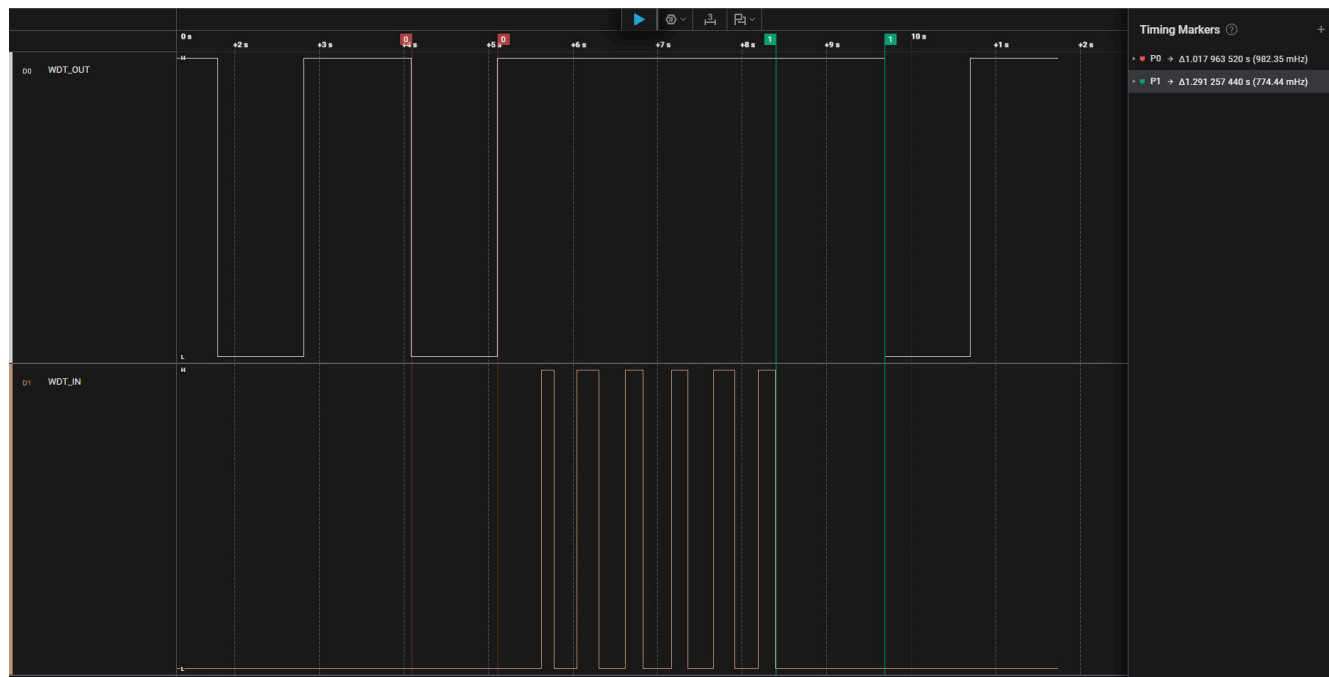
Figure 3. WDT With Longer Output Assertion Time
