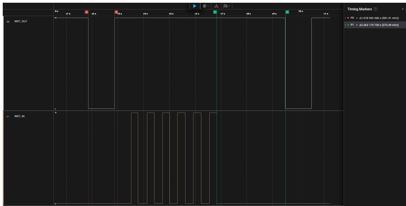
Figure 4. WDT With Longer Timeout Period and Longer Output Assertion Time
