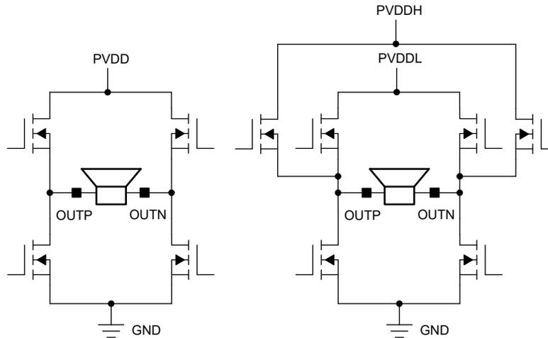
**Figure 1. Traditional Class-D Amplifier vs Simplified Y-Bridge Architecture**
