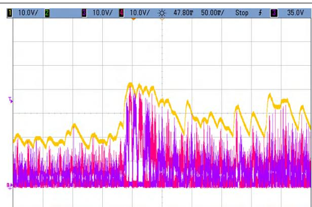
**Figure 3. Audio Output and Boost Voltage With Class-H Operation**
