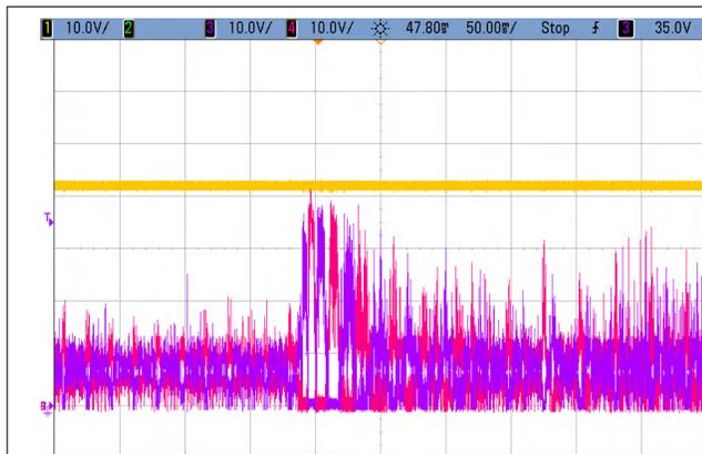
**Figure 2. Audio Output and Boost Voltage Without Class-H Operation**
