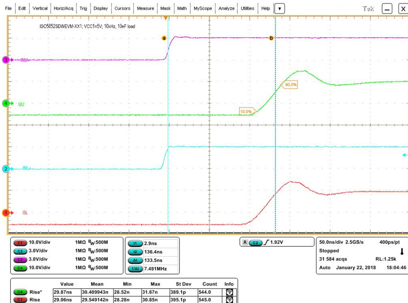
Figure 20. Rise Time and Propagation Delay Waveforms with 10 nF Load
