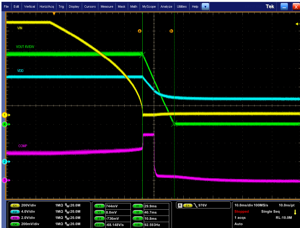
Figure 5-14. Shutdown, VIN Removal: VIN = 1000 V, Load = 2.7 A
