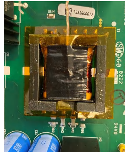
Figure 5-37. Black tape for thermal camera
