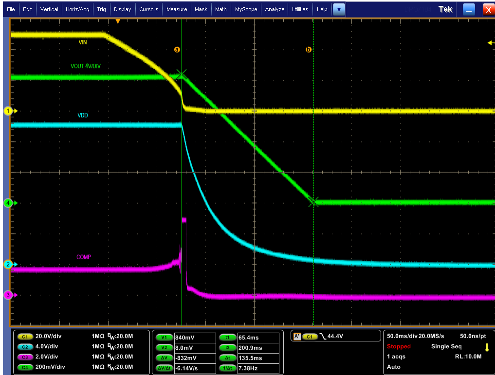
Figure 5-11. Shutdown, VIN Removal: VIN = 50 V, Load = 0.25 A
