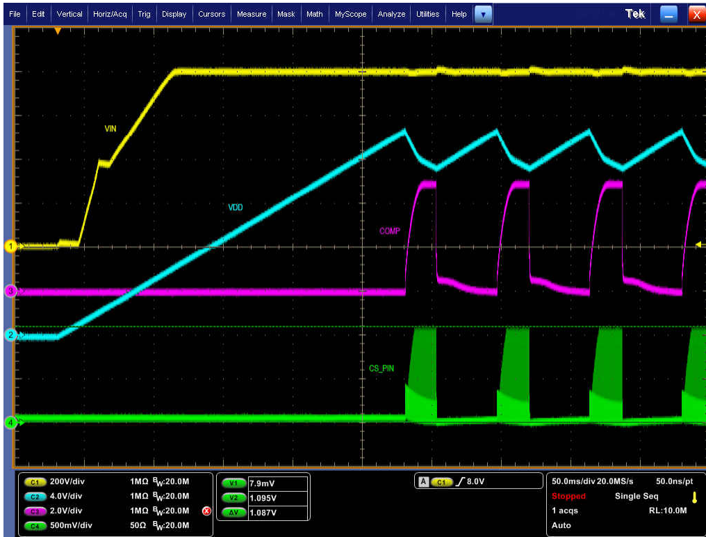
Figure 5-29. 800 VIN, Startup with output shorted to ground
