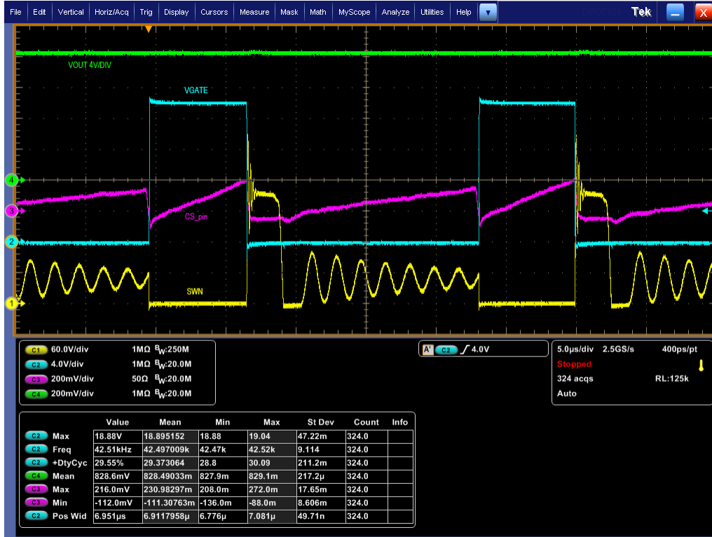
Figure 5-19. Steady State: VIN = 50 V, Load = 0.25 A
