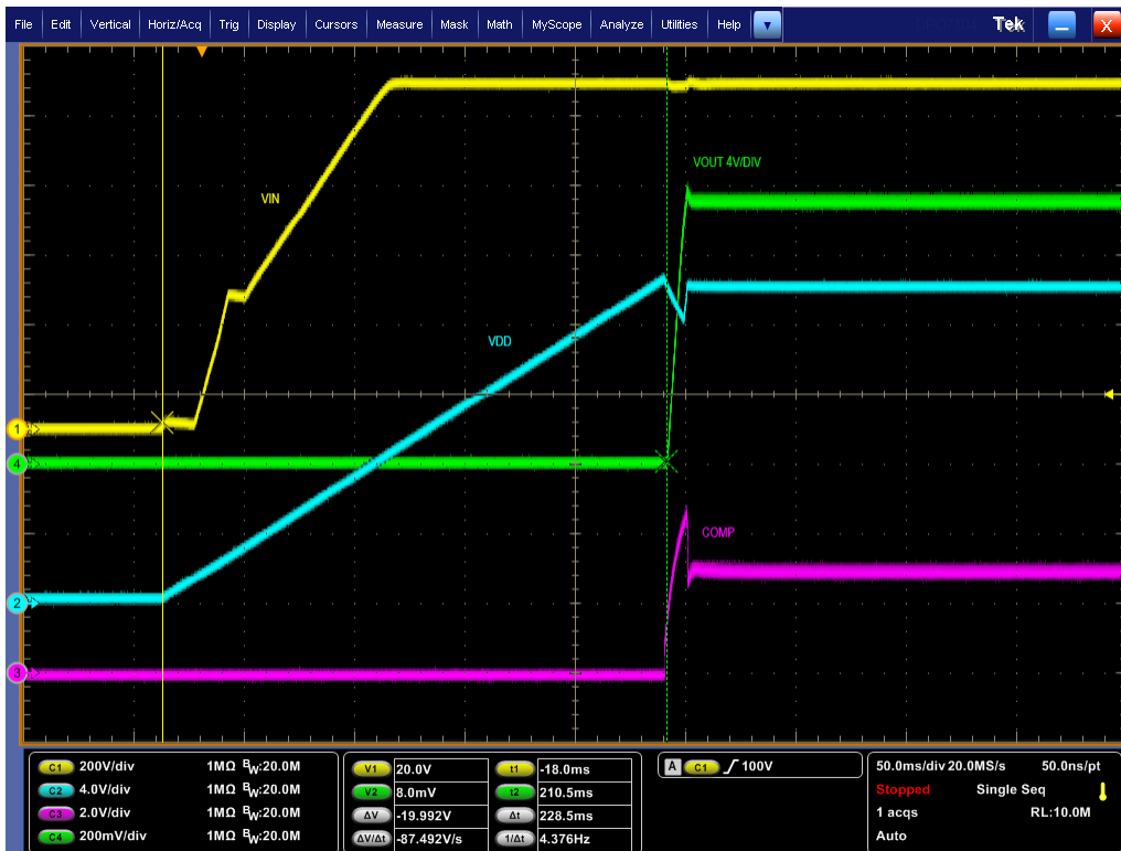
Figure 5-10. Start-Up 4: VIN = 1000 V, Load = 2.7 A
