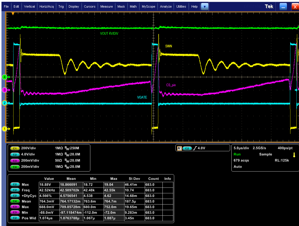
Figure 5-22. Steady State: VIN = 1000 V, Load = 2.7 A
