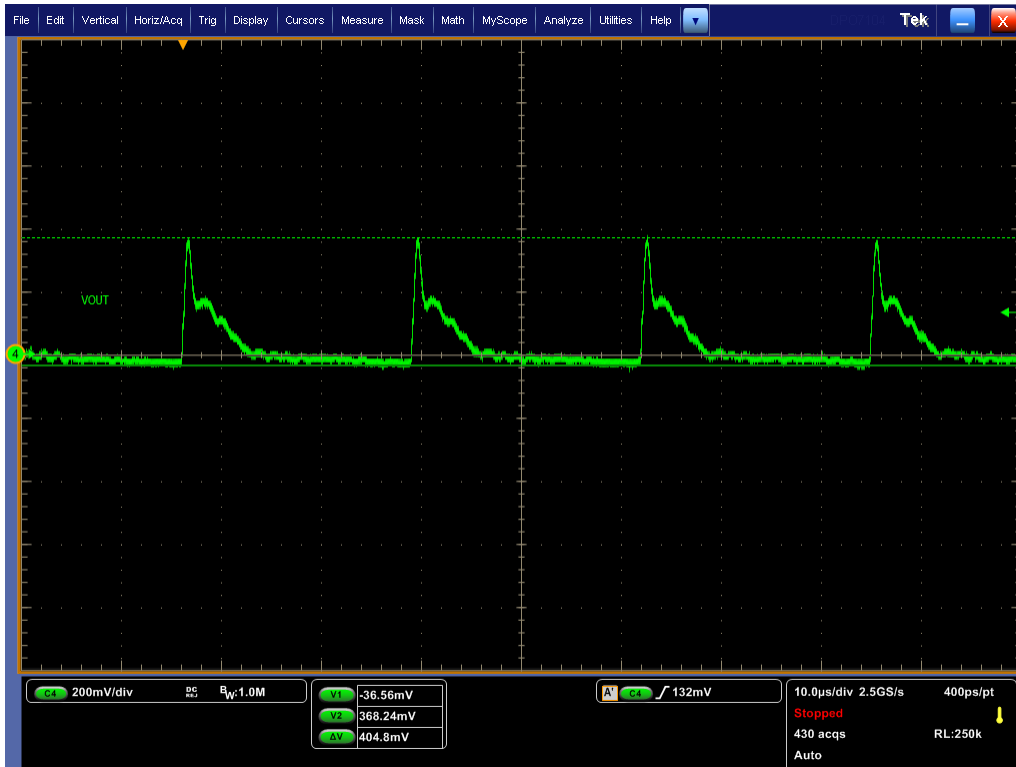
Figure 5-18. Output Voltage Ripple: VIN = 1000 V, Load = 2.7 A
