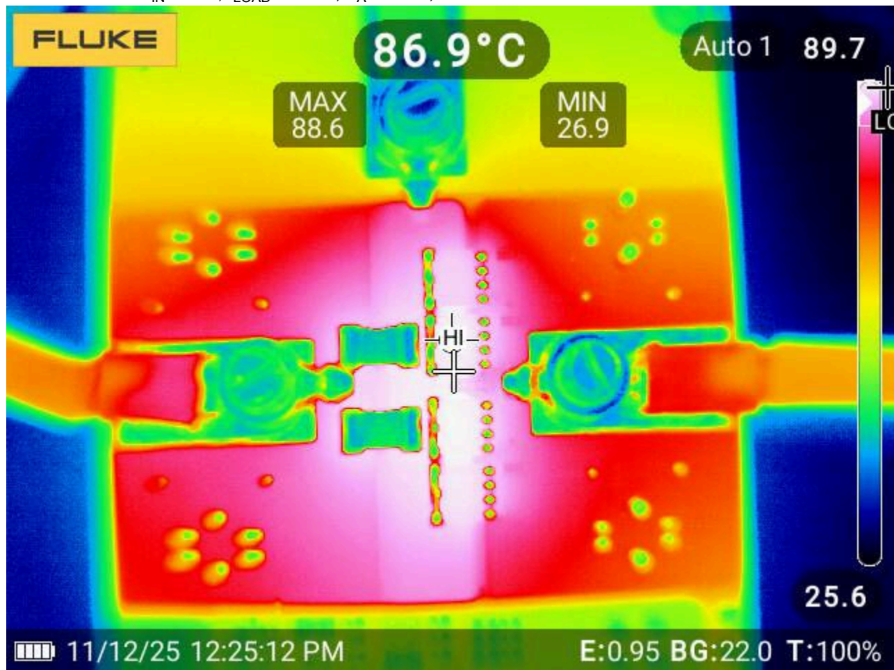
Figure 3-32. Thermal Performance of LM5066H1EVM
