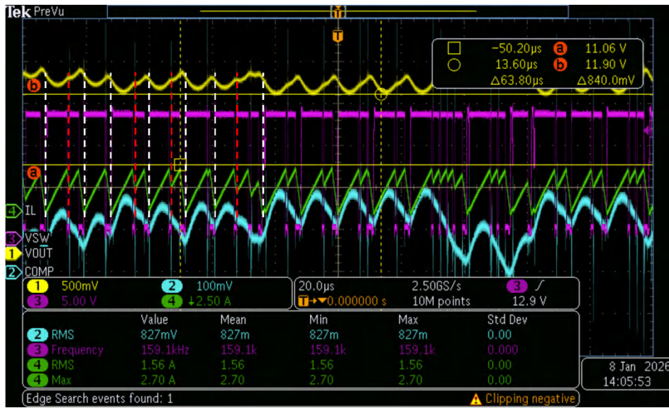
Figure 4-2. Experimental Results of LM5190 at a Load Current of 0.991A
