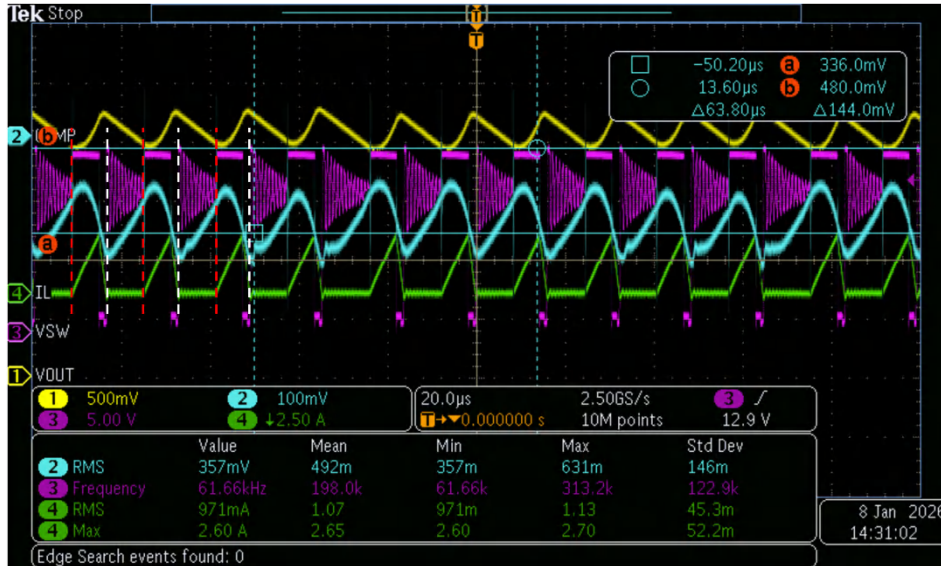
Figure 5-1. Experimental Results of LM5190 at a Load Current of 0.589A
