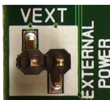
Figure 11 – TrxEB rev. 1.7.0 external power supply header (P1)
