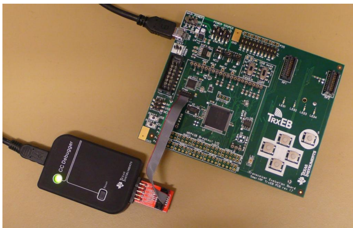
Figure 33 – Proper connection for board resurrection.
