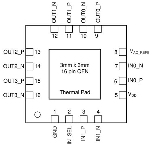
Figure 6-1. LMK1D1204: RGT Package 16-Pin VQFN Top View
