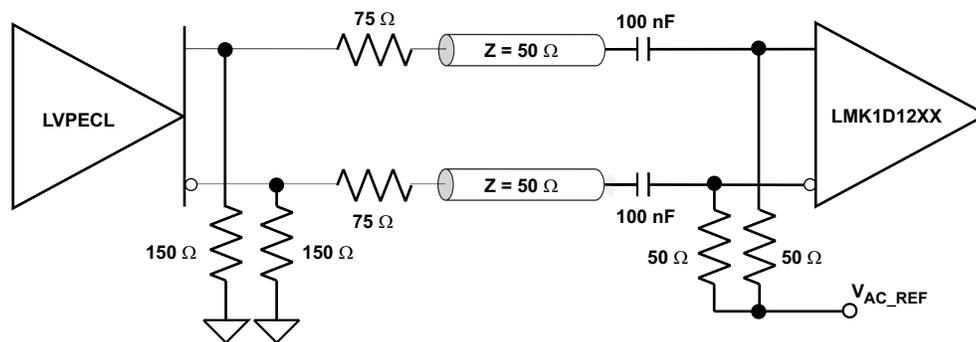
**Figure 9-5. LVPECL Clock Driver Connected to LMK1D120x Input**
