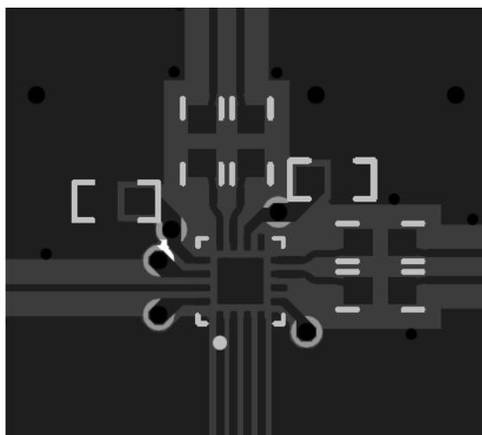
**Figure 9-9. PCB Layout Example for LMK3H0102, Top Layer**
