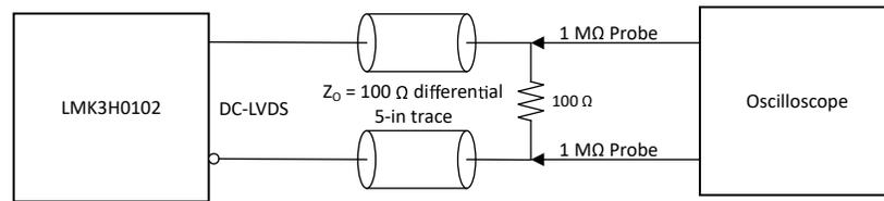
Figure 7-3. DC-LVDS Output Configuration During Device Test
