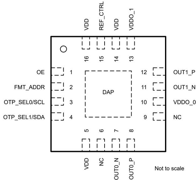
Figure 4-1. LMK3H0102 16-Pin VQFN Top View
