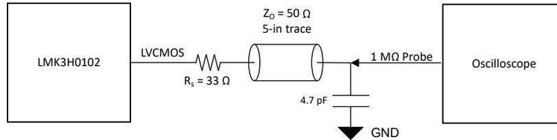
Figure 7-1. LVCMOS Output Configuration During Device Test
