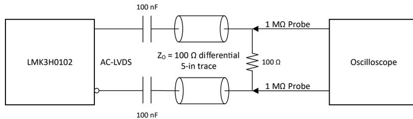
Figure 7-2. AC-LVDS Output Configuration During Device Test
