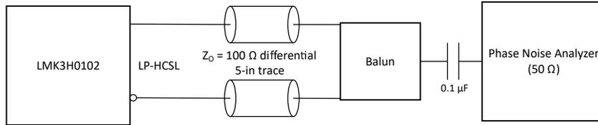
**Figure 7-6. PCIe Test Configuration Using Phase Noise Analyzer**
