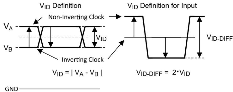
Figure 6-1. Two Different Definitions for Differential Input Signals
