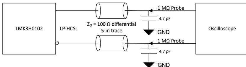
Figure 7-4. LP-HCSL Output Configuration During Non-PCIe Device Test
