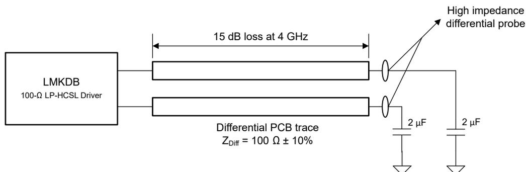
Figure 7-5. LP-HCSL Output Configuration During PCIe Device Test
