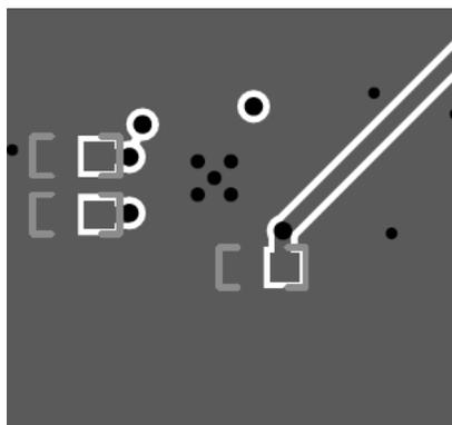
**Figure 9-10. PCB Layout Example for LMK3H0102, Bottom Layer**
