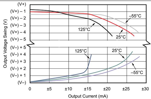
Figure 16. Output Voltage Swing vs Output Current
