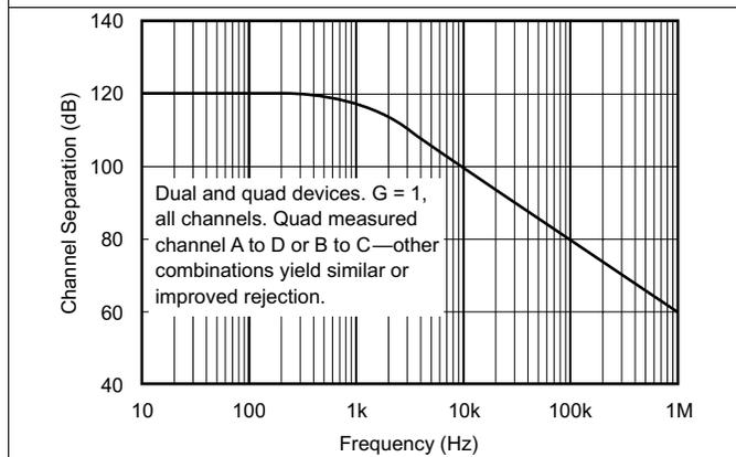
Figure 5. Channel Separation vs Frequency
