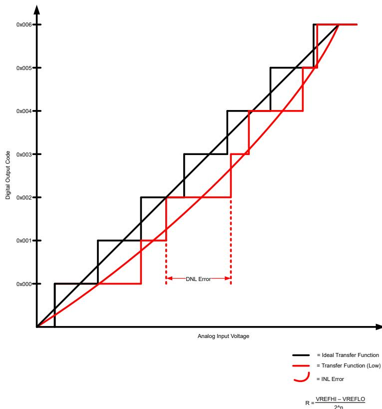
**Figure 6-36. ADC INL and DNL****6.14.4.2.4 ADC Input Model****Table 6-16. Input Model Parameters**
