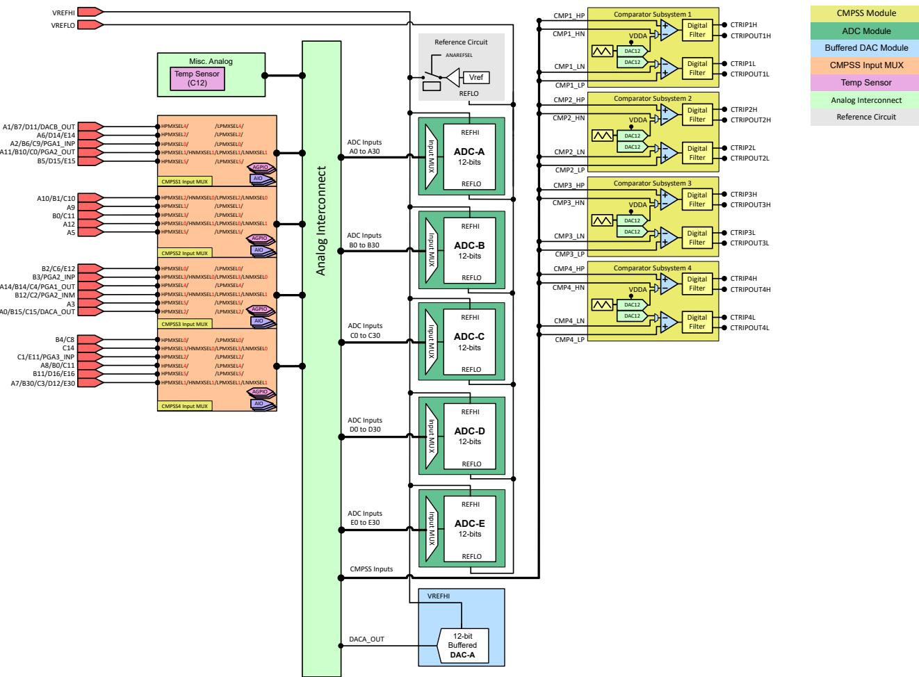
**Figure 6-32. Analog Subsystem Block Diagram (100-Pin Package)**
