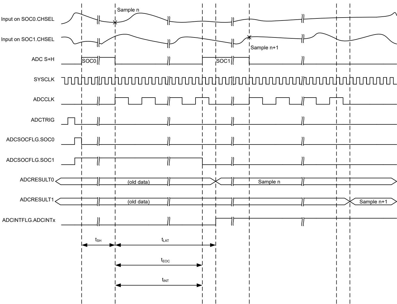
Figure 6-39. ADC Timings for 12-bit Mode in Late Interrupt Mode
