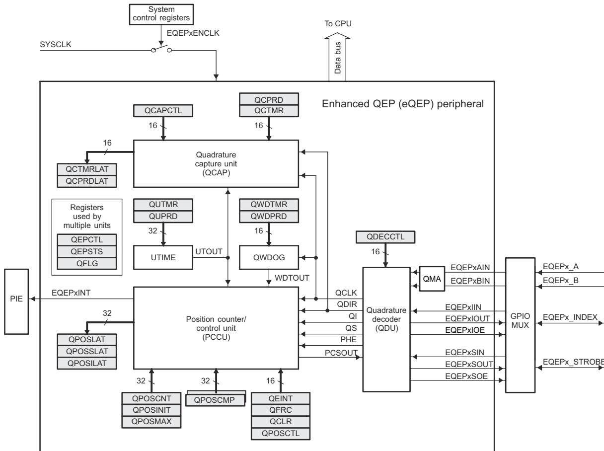
**Figure 6-57. eQEP Block Diagram**
