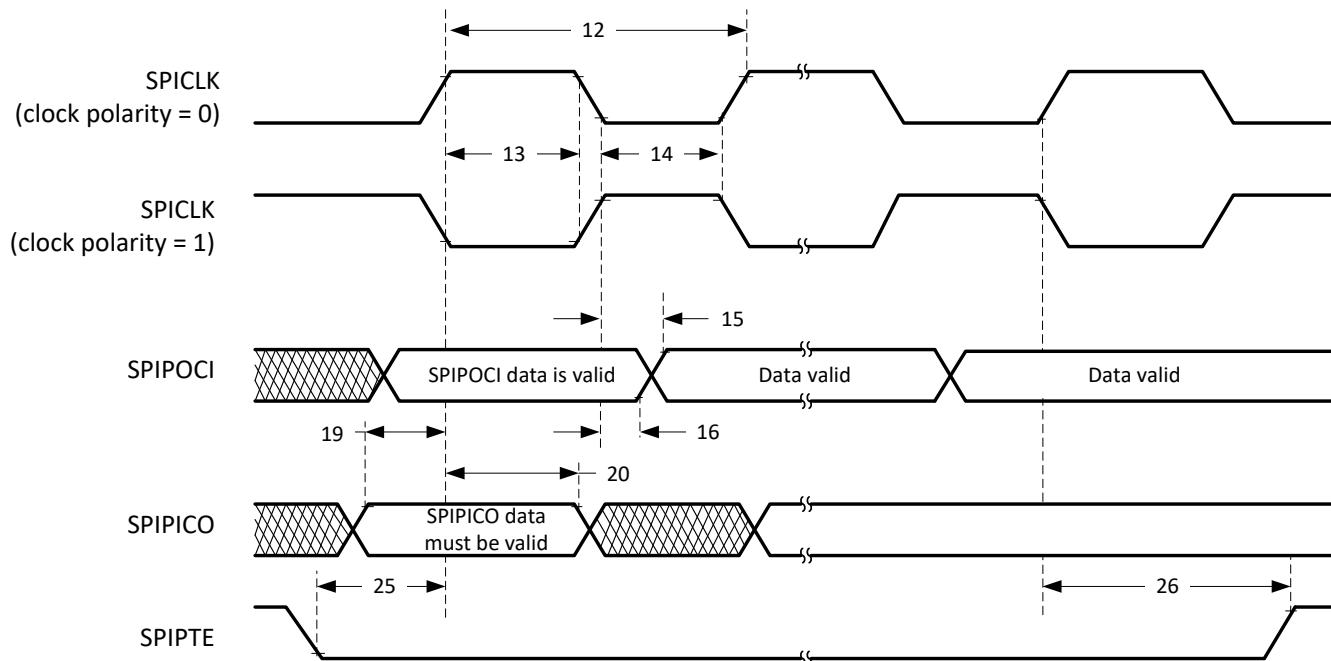
Figure 6-67. SPI Peripheral Mode External Timing (Clock Phase = 1)
