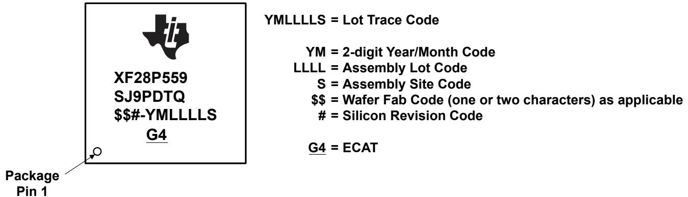
**Figure 9-2. Package Symbolization for PDT Package – Automotive**
