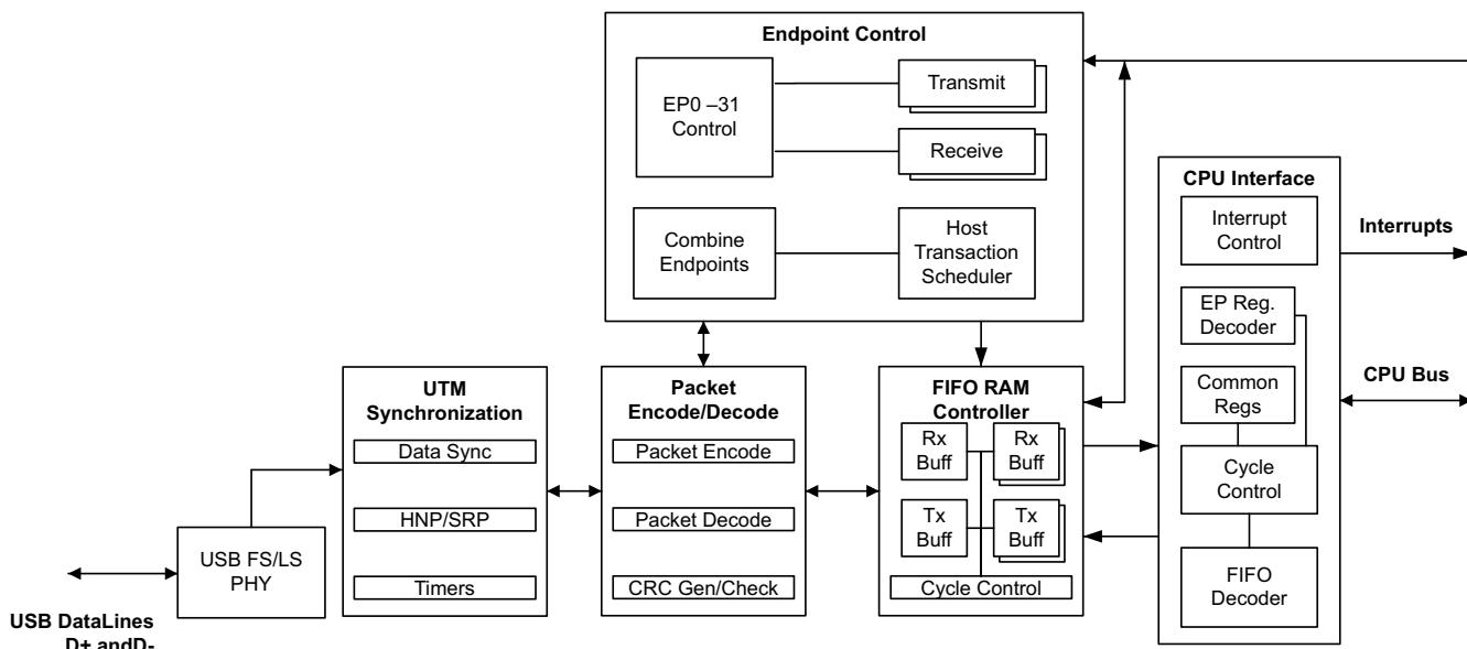
**Figure 6-76. USB Block Diagram**
