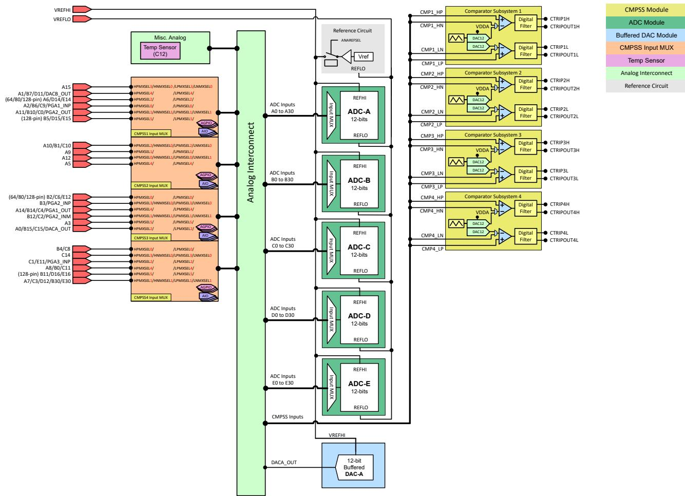
**Figure 6-31. Analog Subsystem Block Diagram (128-/80-/64-/56-Pin Packages)**
