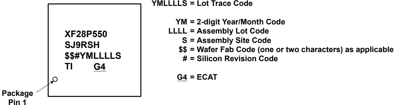
**Figure 9-9. Package Symbolization for RSH Package – Non-Automotive**
