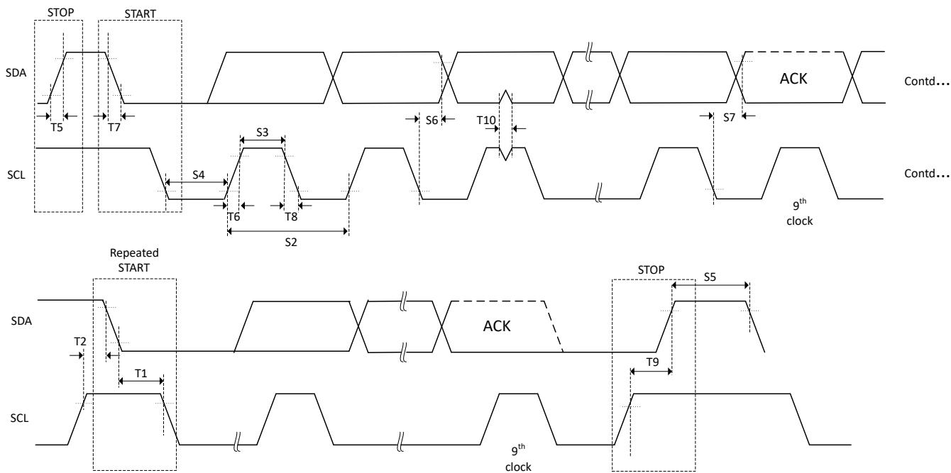
Figure 6-60. I<sub>2</sub>C Timing Diagram
