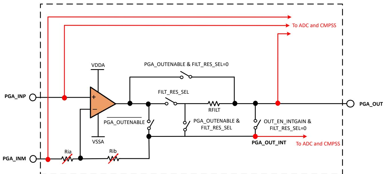
**Figure 6-49. PGA Block Diagram**
