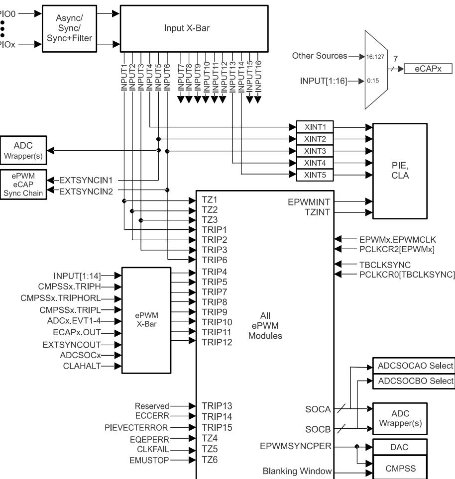
Figure 6-51. ePWM Trip Input Connectivity
