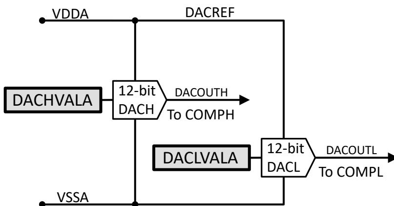
**Figure 6-42. Reference DAC Block Diagram**
