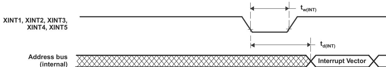
Figure 6-27. External Interrupt Timing
