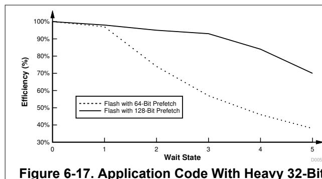
**Figure 6-17. Application Code With Heavy 32-Bit Floating-Point Math Instructions**
