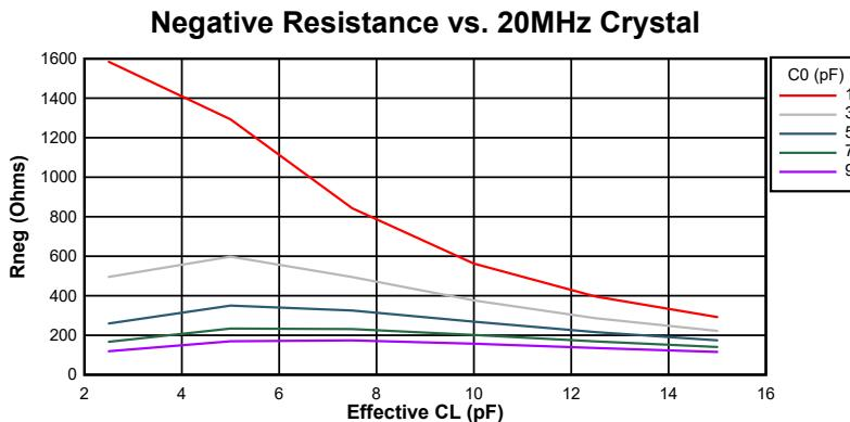
**Figure 6-16. Negative Resistance Variation at 20 MHz****ADVANCE INFORMATION****6.13.3.4.7.3 Crystal Oscillator Parameters**
