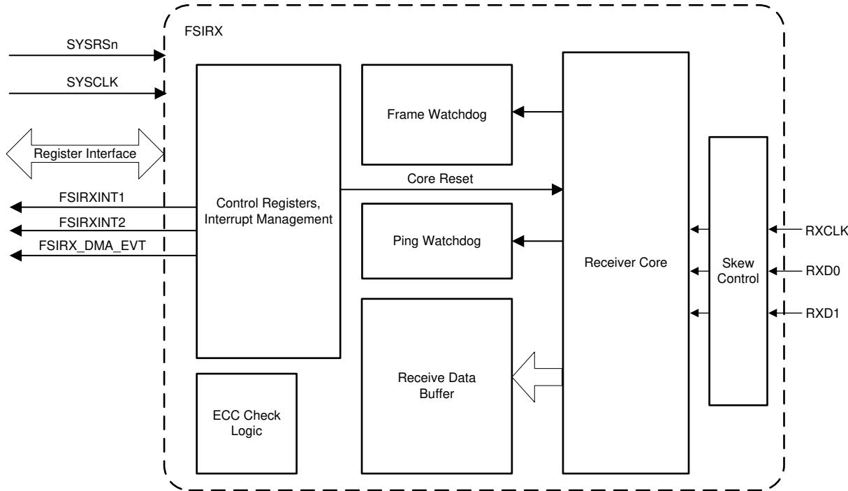
**Figure 6-73. FSIRX Block Diagram****6.16.7.2.1 FSIRX Electrical Data and Timing****6.16.7.2.1.1 FSIRX Timing Requirements**
