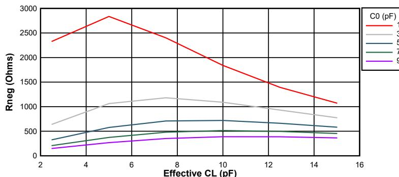
**Figure 6-15. Negative Resistance Variation at 10 MHz**
