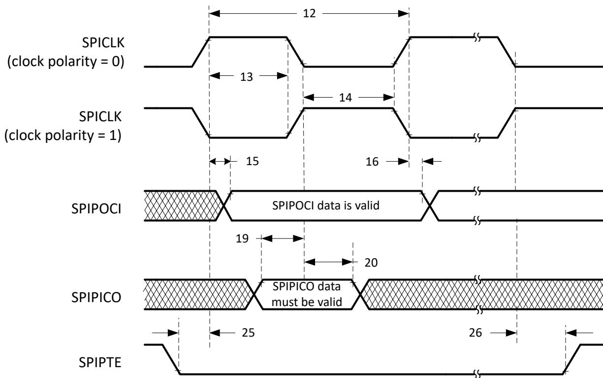
Figure 6-66. SPI Peripheral Mode External Timing (Clock Phase = 0)
