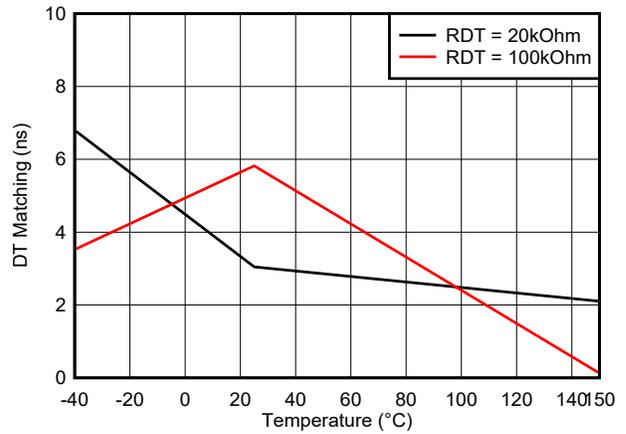
Figure 5-23. Dead Time Matching vs Temperature (with R<sub>DT</sub> = 20kΩ and 100kΩ)
