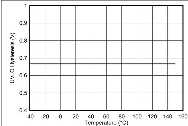
Figure 5-18. VDD 8-V UVLO Hysteresis vs Temperature
