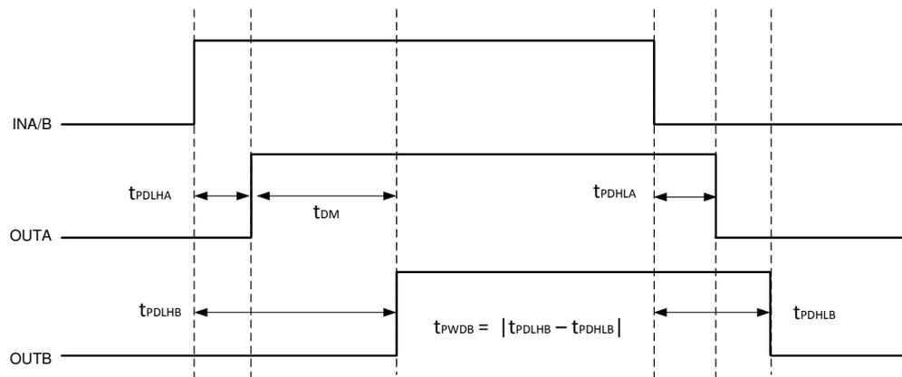
Figure 6-3. Delay Matching and Pulse Width Distortion
