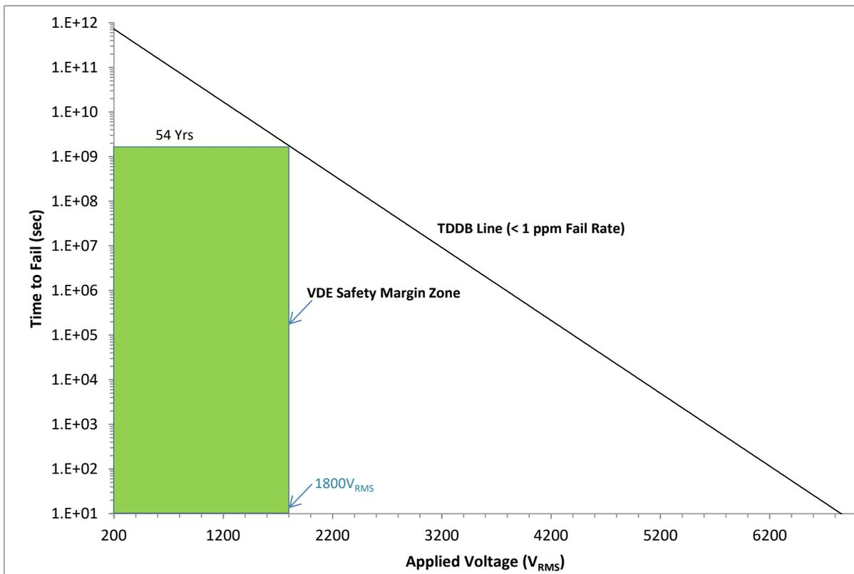
**Figure 5-3. Reinforced Isolation Capacitor Life Time Projection**
