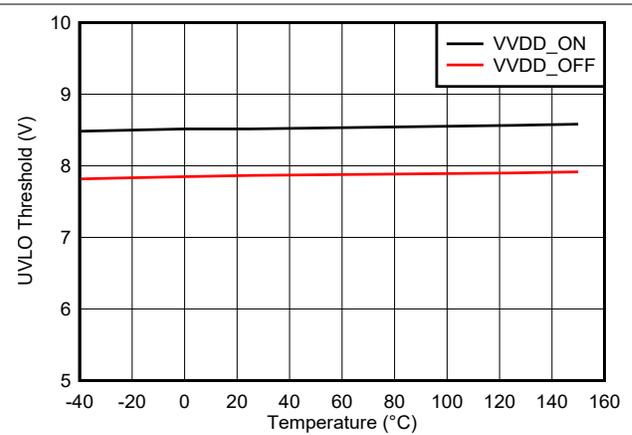
Figure 5-17. VDD 8-V UVLO Threshold vs Temperature
