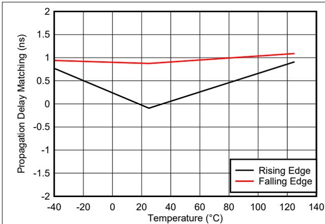
Figure 5-16. Propagation Delay Matching (t<sub>DM</sub>) vs Temperature
