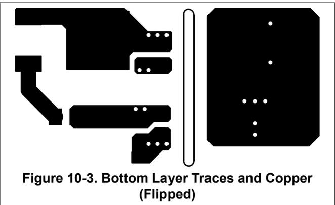
Figure 10-3. Bottom Layer Traces and Copper (Flipped)
