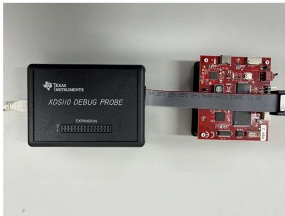
**Figure 3-3. XDS110 Debug Probe and Board Assembly**
