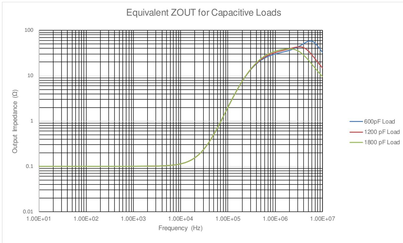
Figure 4-3.  $Z_{EQ}$  for Various  $C_{FILT}$
