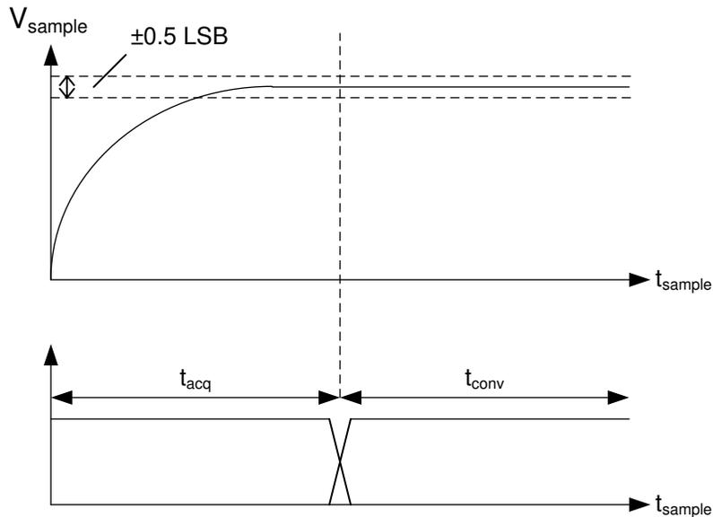
Figure 2-1. Typical ADC Single Acquisition Cycle
