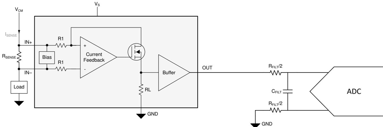
**Figure 3-1. Charge Bucket Filter, Single-Ended ADC with Ground Sense Configuration**
