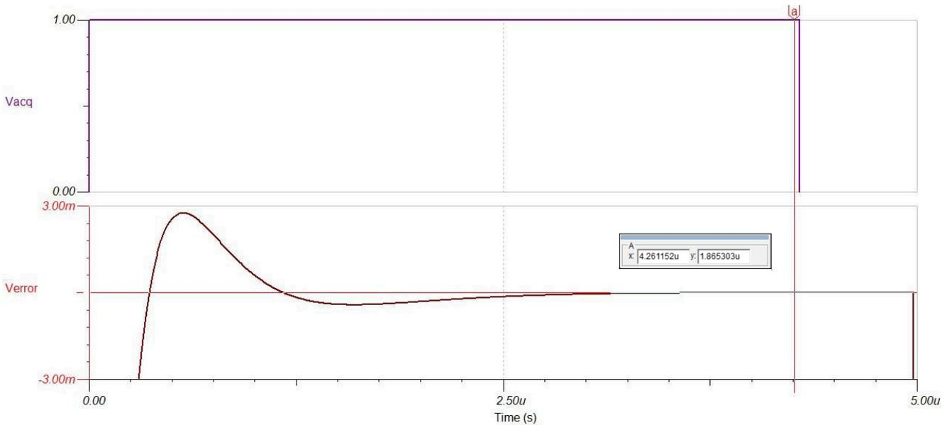
Figure 4-9. ADS8860 Error Response,  $f_{\text{sample}} = 200\text{kHz}$ ,  $R_{\text{FILT}} = 104.4\Omega$
