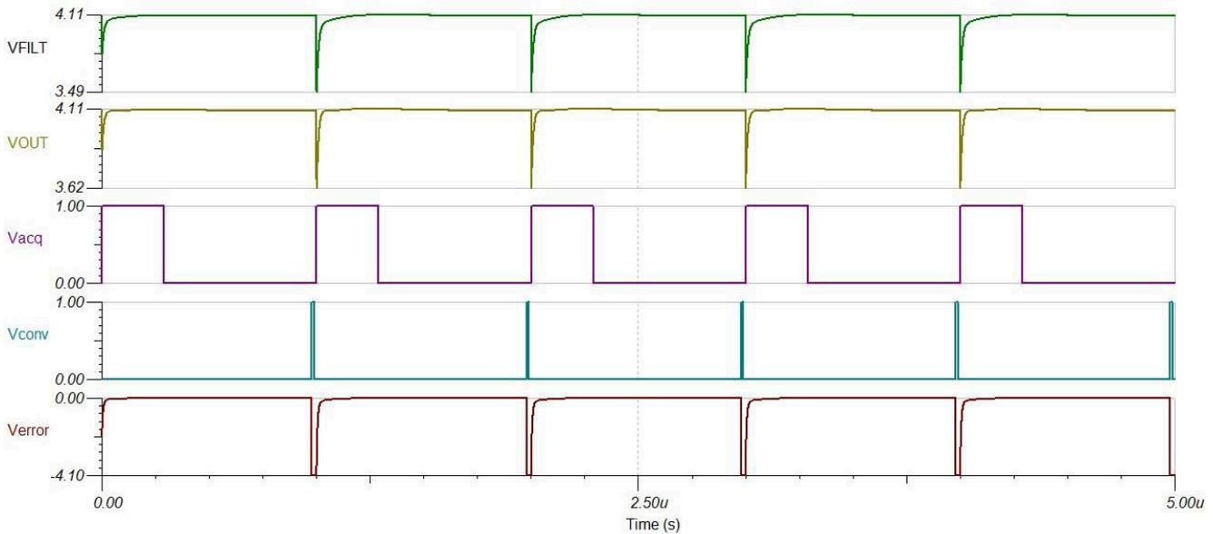
**Figure 4-7. Sample and Hold Initial Waveforms**
