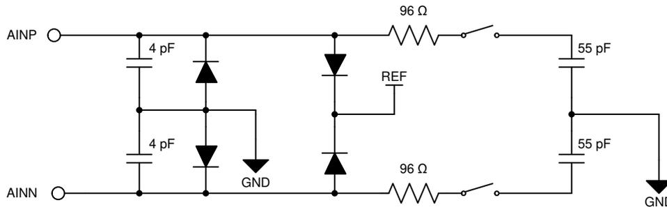
Figure 2-2. ADS8860 Input Sampling Stage Equivalent Circuit, Hold Mode
