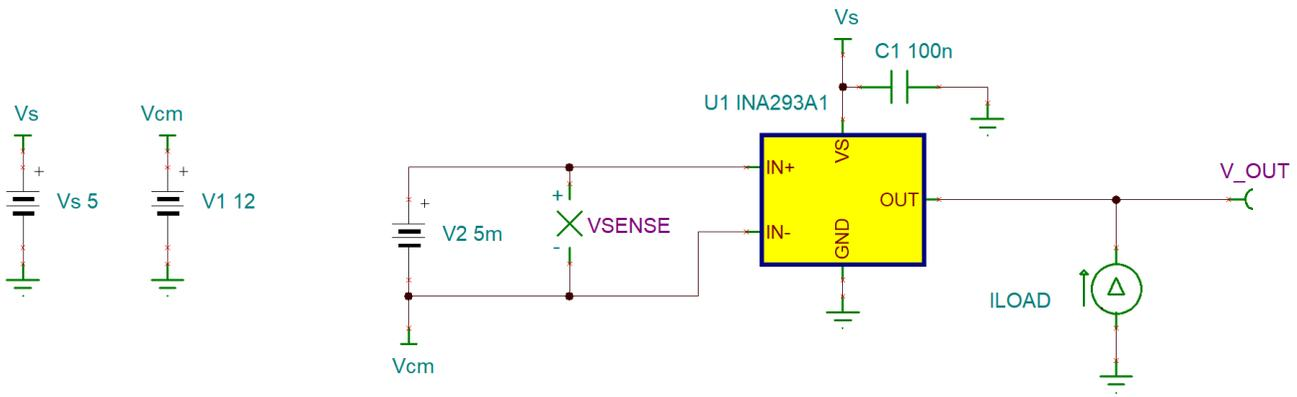
Figure 4-1. INA293  $Z_{OUT}$  Test Circuit
