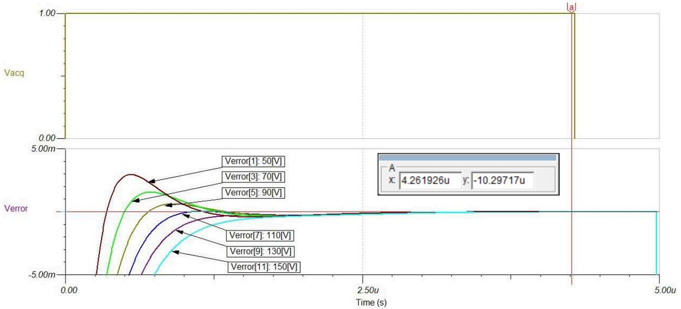
Figure 4-10. Effects of  $R_{FILT}$  on Error Response
