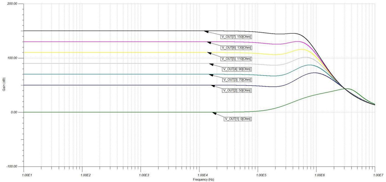
Figure 4-11. AC Response of INA293 With Various  $R_{FILT}$
