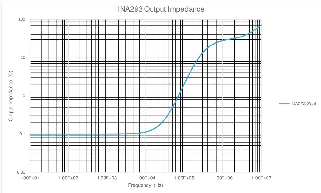
Figure 4-2. INA293  $Z_{OUT}$  Output Impedance
