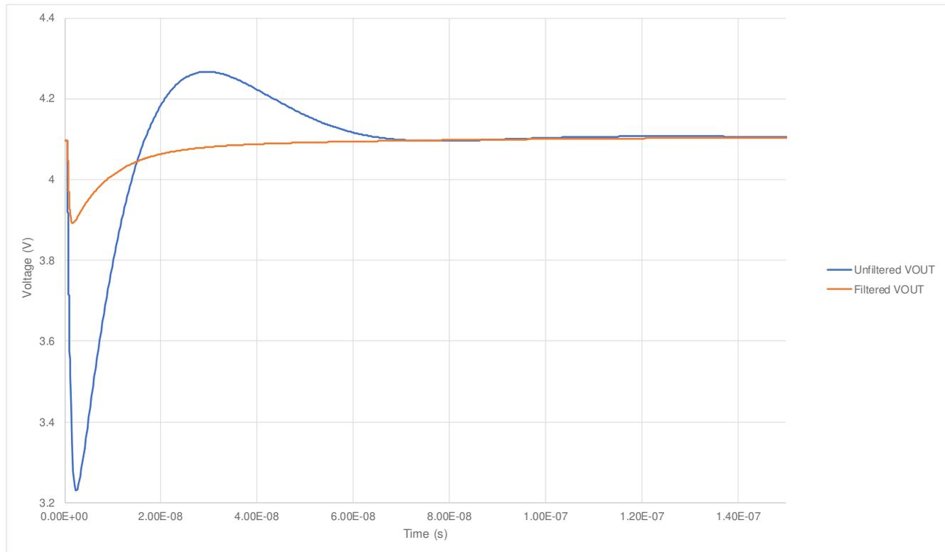
**Figure 3-2. Unfiltered vs. Filtered Output Signal**
