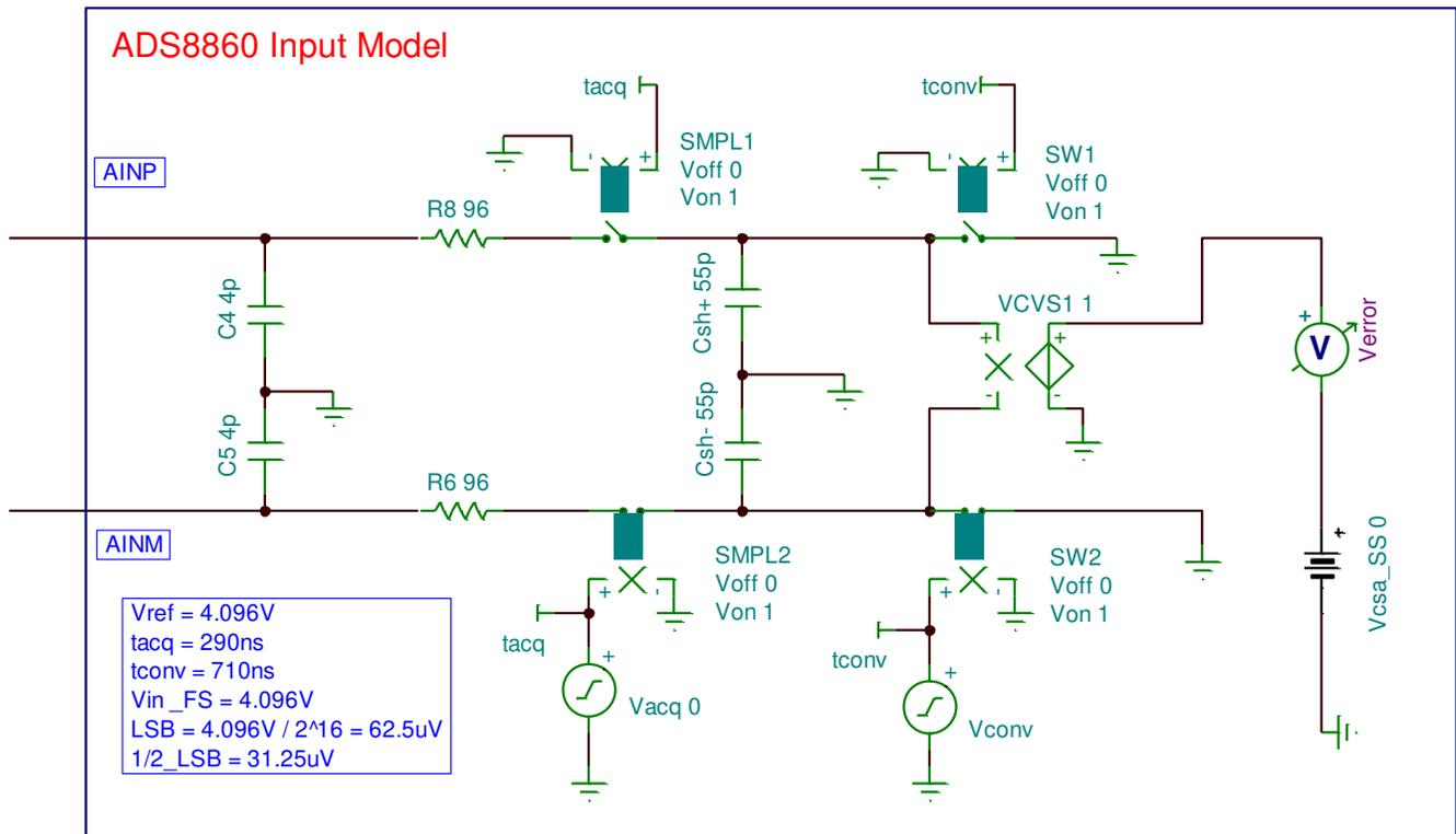
**Figure 4-4. ADS8860 Switching Simulation Model**
