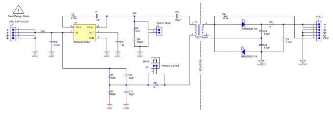
Figure 1-2. Schematic of Design 2
