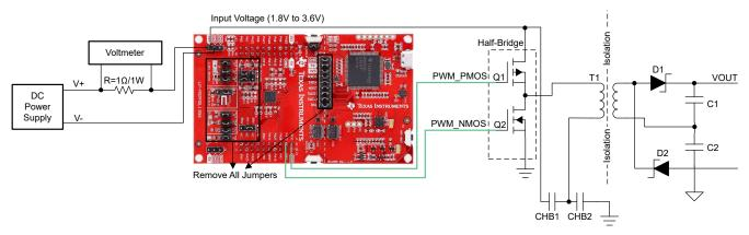
Figure 1-4. Set Up of Current Consumption Test on MSPM0L1306 EVM Board
