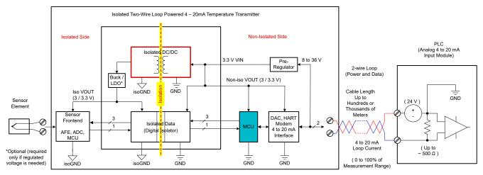
Figure 1-1. Isolated Two-Wire Loop-Powered 4 to 20mA Temperature Transmitter Control System
