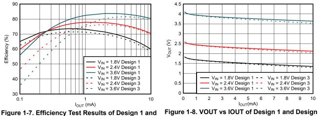
Design 3 at 50khz Switching Frequency
