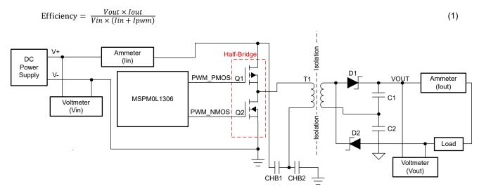
Figure 1-6. Set Up of Efficiency Test
