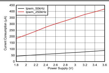
Figure 1-5. Current Consumption versus Power Supply Voltage at Different PWM Frequency of MSPM0L1306
