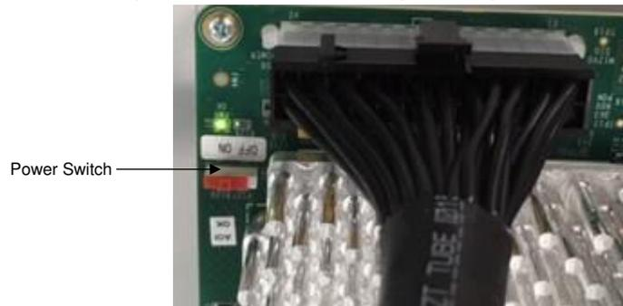
**Figure 6-4. Alpha Data Board Power Switch**
