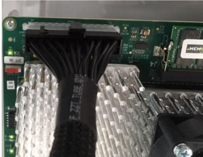
**Figure 6-2. Output Power Cable Connection**
