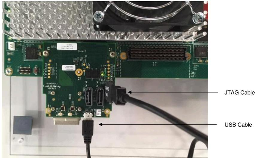
**Figure 6-3. JTAG and USB Cable Connections**
