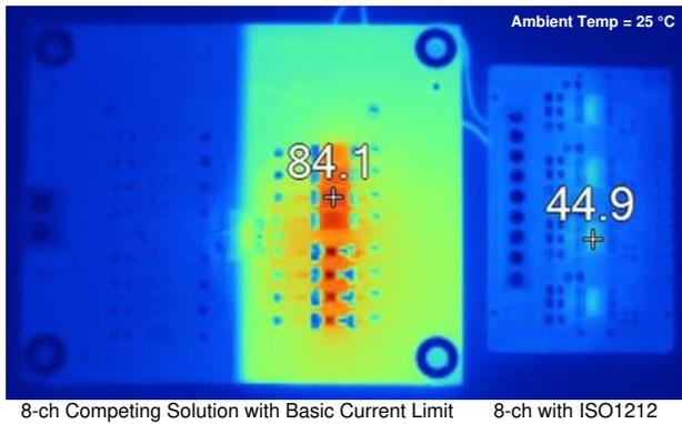
**Figure 3. Board temperature comparison: Traditional solution vs ISO1212**
