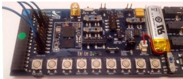
Figure 11. Figure 8. Control Buttons on CSR Board
