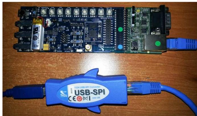
**Figure 2. CSR Programming Setup**
