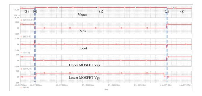
Figure 3-6. Simulation Results (D=50%, C<sub>boot</sub>=100nF)
