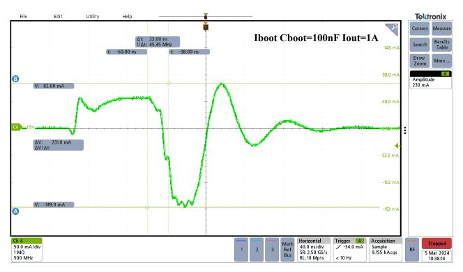
Figure 3-12. Experiment Results (100nF Bootstrap Capacitor)
