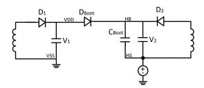
Figure 3-9. Schematic With V<sub>2</sub> Connected
