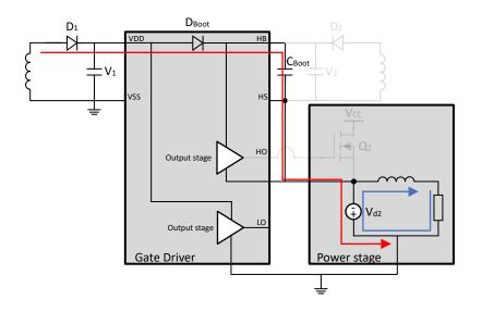
Figure 3-4. Equivalent Circuit in Mode 2
