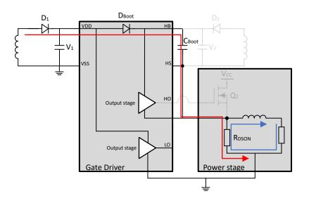
Figure 3-3. Equivalent Circuit in Mode 1
