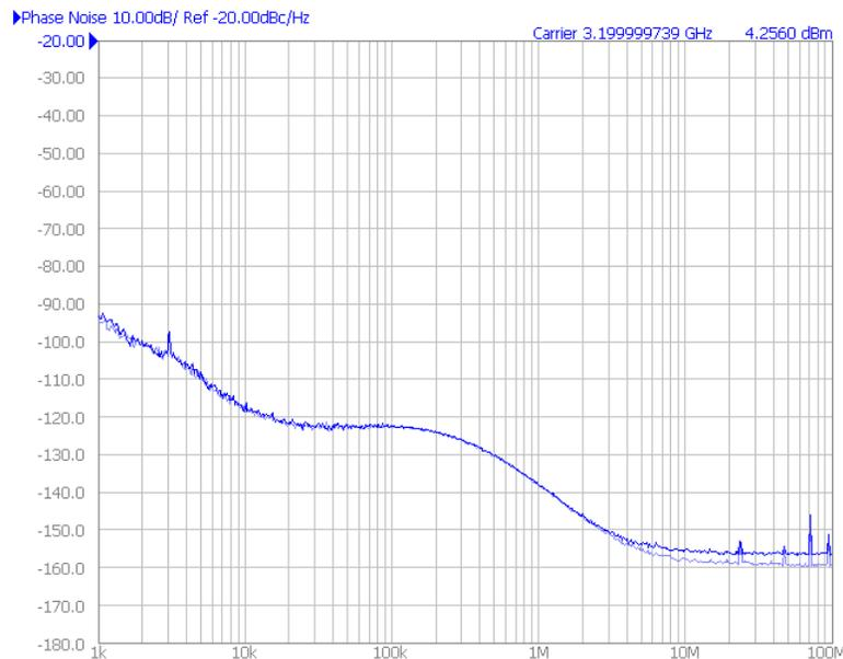
**Figure 4-2. 3200MHz Buffer Mode Signal Analyzer Plot**
