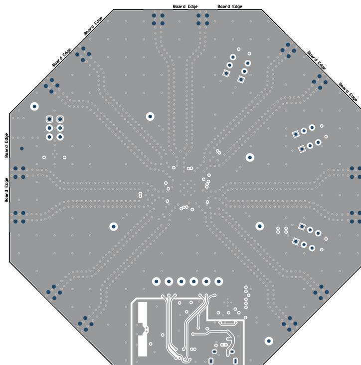
**Figure 5-5. Layer 2 (RF GND)**
