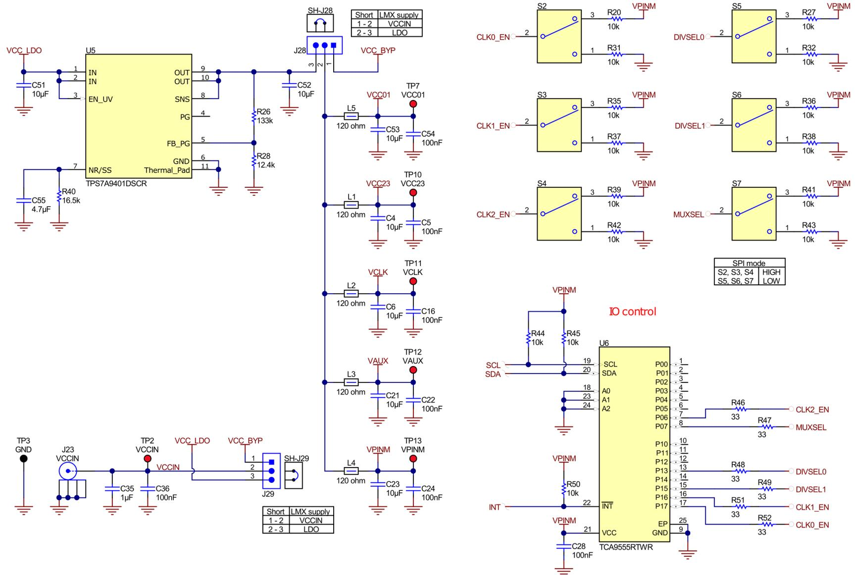
Figure 5-1. Power Supply, IO Control, Switches
