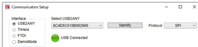
**Figure 3-6. Identify USB2ANY Controller**
