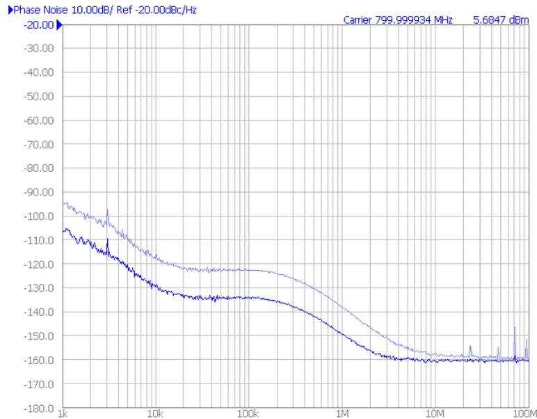
**Figure 4-3. 3200MHz Divide by 2 Mode Signal Analyzer Plot**
