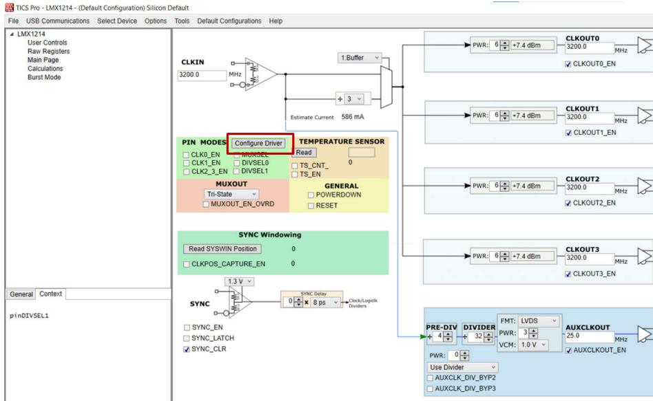
Figure 2-4. How to Configure IO Expander
