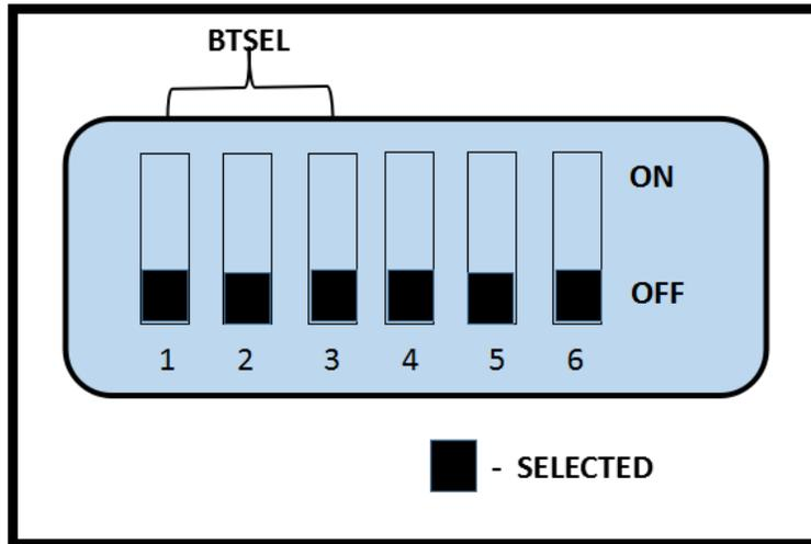
2. Verify DIP SW5 is configured to 1.35-V core voltage mode and component video output mode.
