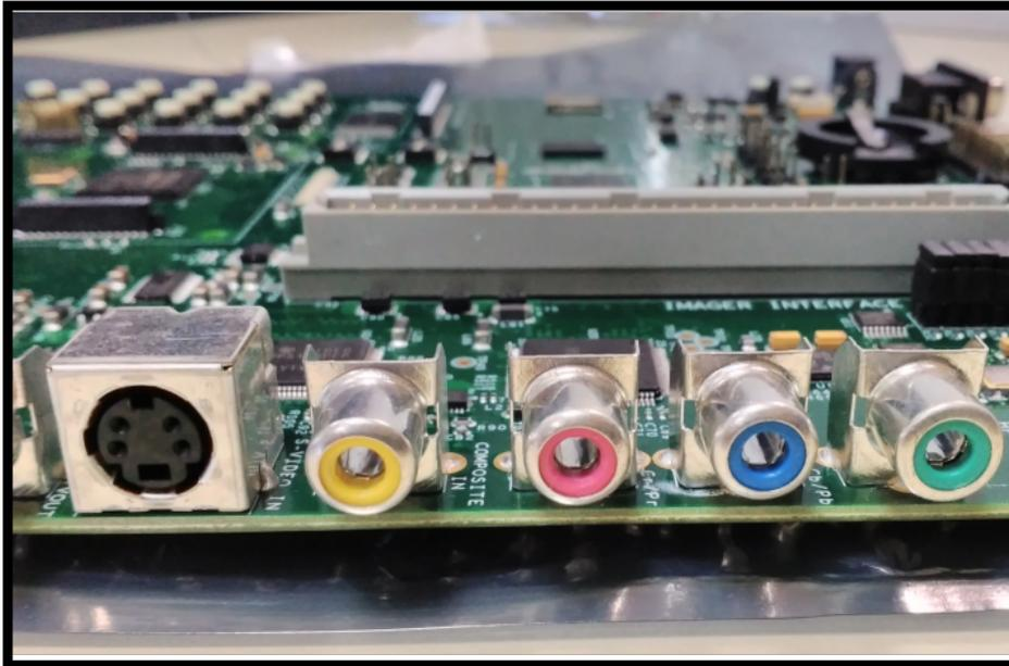
4. Connect your HD video display to the component video out RCA connector. Power on the HD video display.
