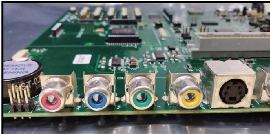
5. Connect an audio speaker to stereo *line out* and an audio source to stereo *line in*.
