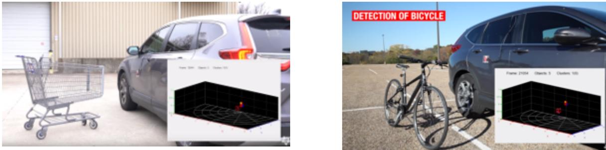
**Figure 5. Detection of Objects with Minimal Surface Area Using the AWR1843AOP EVM**
