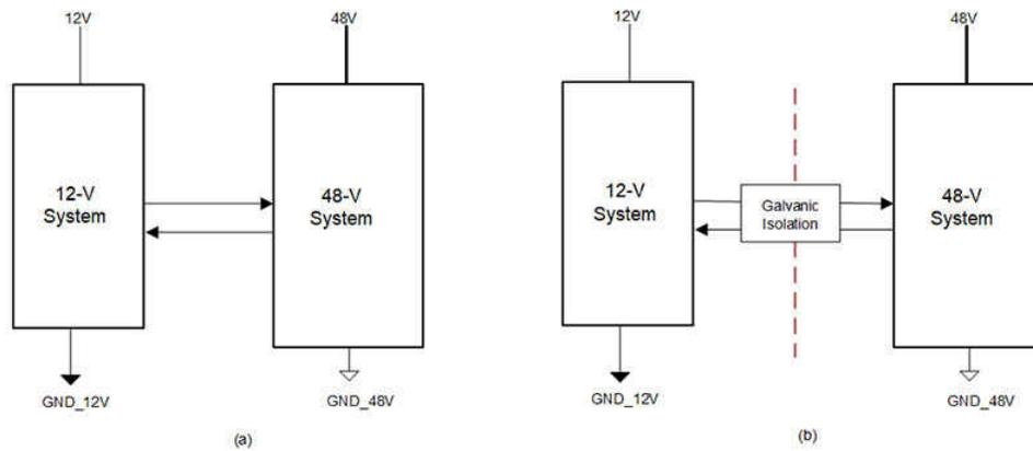
**Figure 1. Direct and Galvanically Isolated Connection between 12-v and 48-v Systems**
