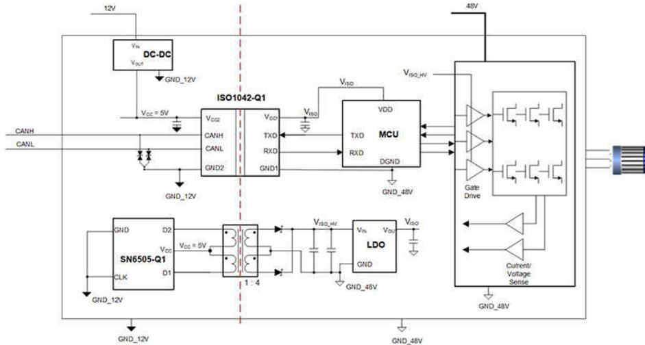
**Figure 3. 48-V Starter Generator Using an Isolated CAN Transceiver with a Push-pull Isolated Power Supply**
