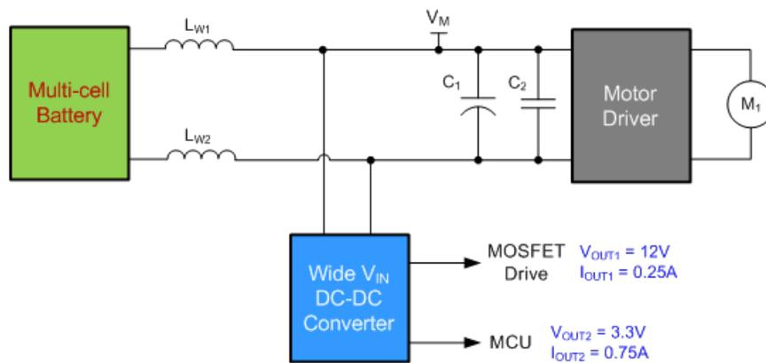
Figure 1. Drone System Block Diagram
