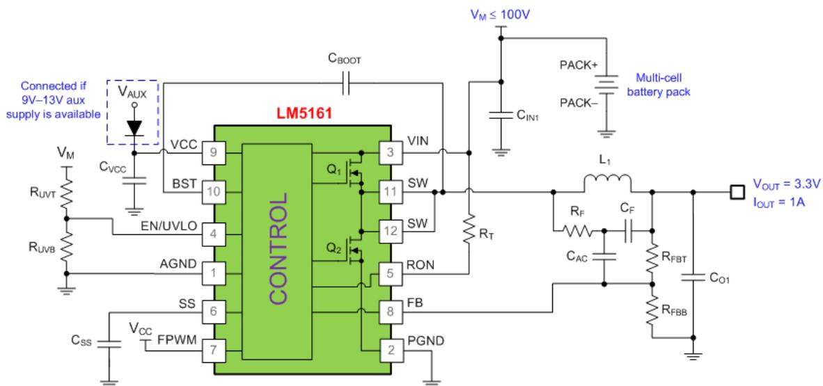
**Figure 3. LM5161 Step-down Converter Schematic**
