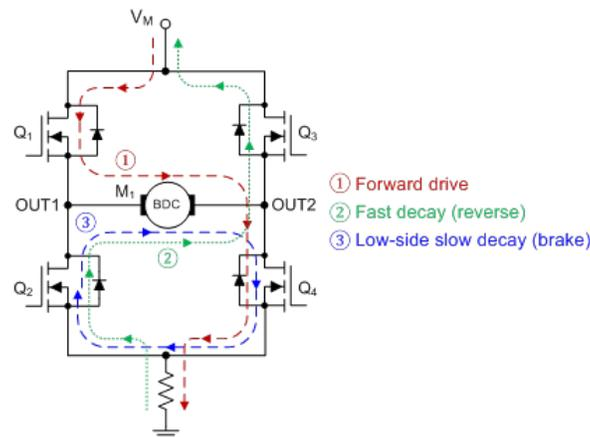
Figure 2. Forward Current Paths of a BDC Motor H-bridge Driver
