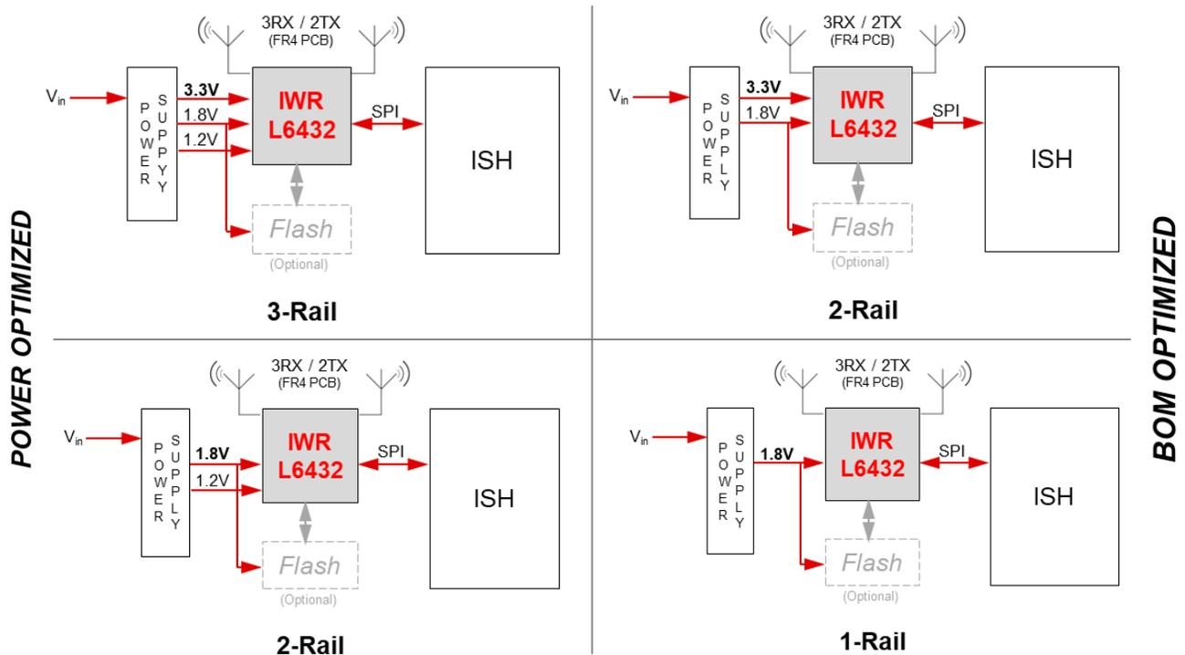
Figure 4-2. IWR L6432 power supply
