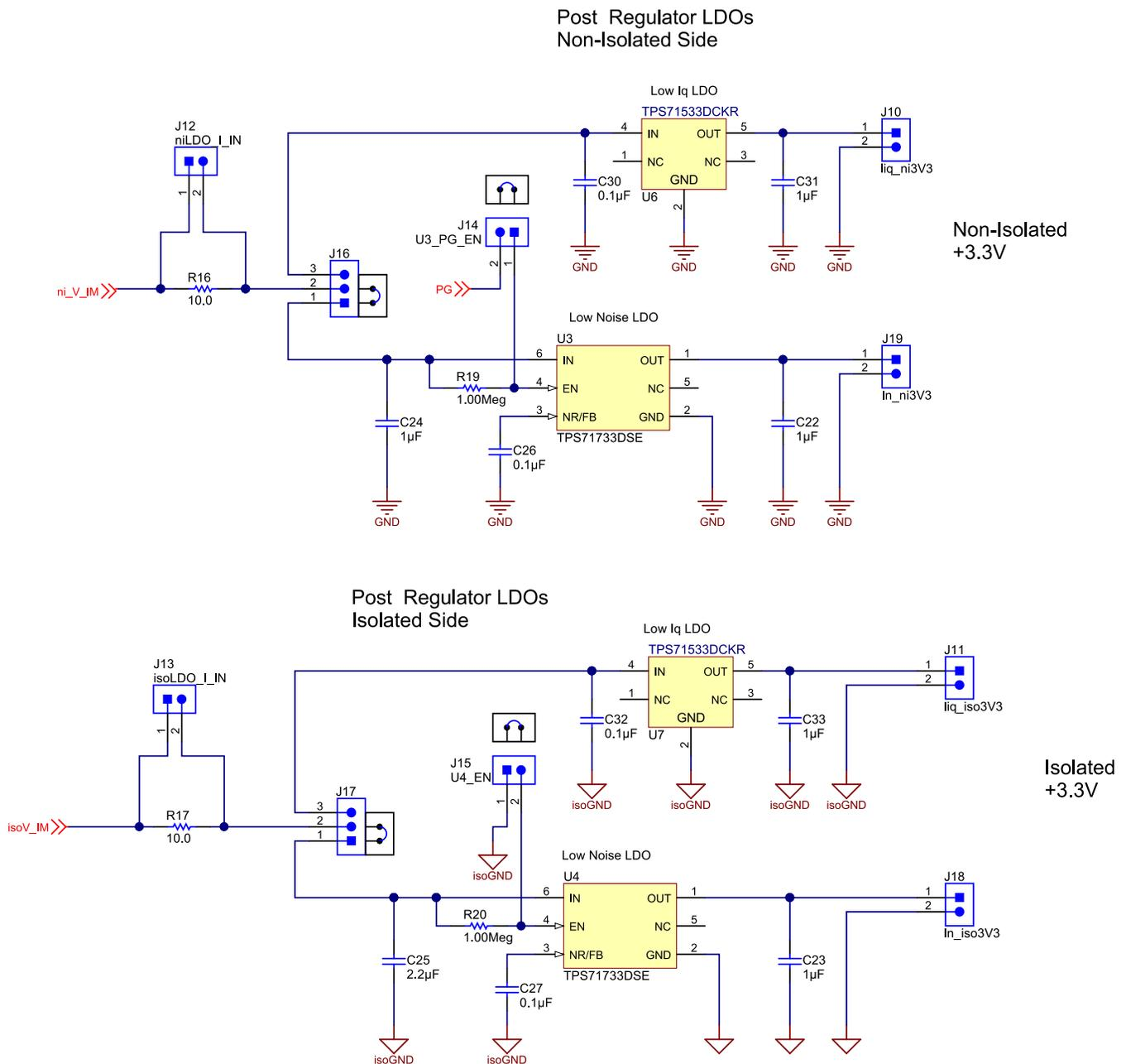
Figure 36. Post-Regulator LDOs — Circuit Implementation
