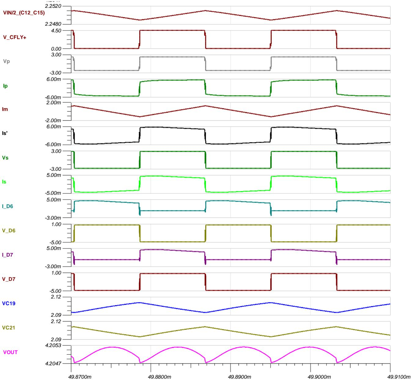
Figure 54. DC/DC Converter — All Waveforms
