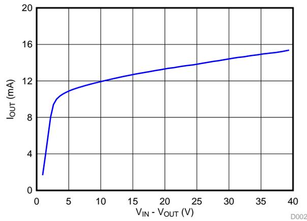
Figure 12. Active Current Limiter Characteristic: IOUT versus VIN-VOUT
