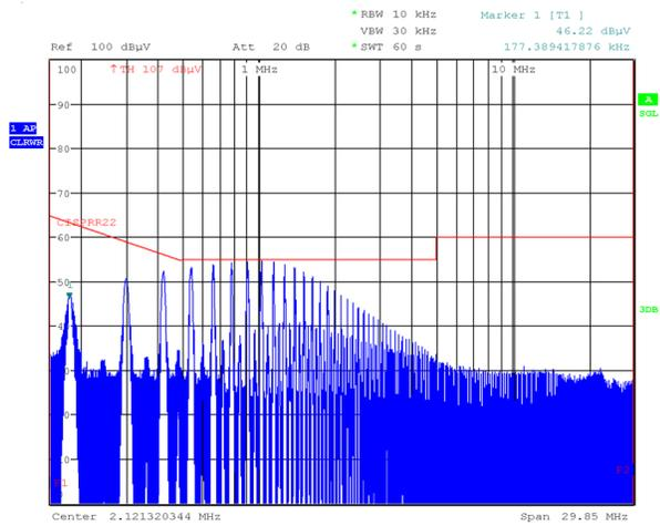
Conducted Noise on "L1", 8V Loop Input, Scaled-Down Ripple Filter, Earthed Load
