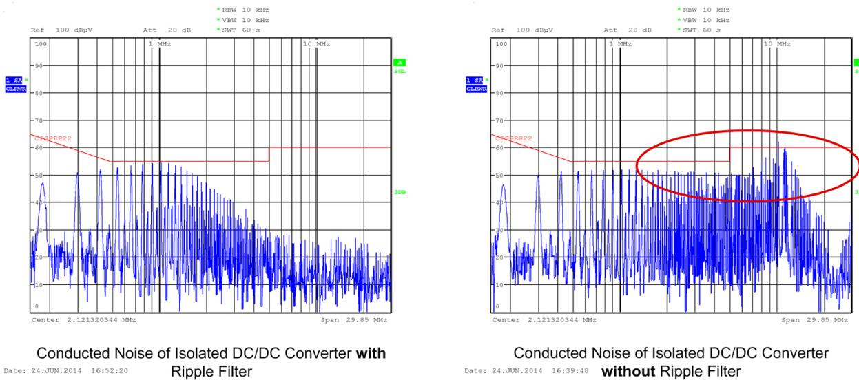
**Figure 27. Conducted Noise of Isolated DC/DC Converter with and without Ripple Filter**
