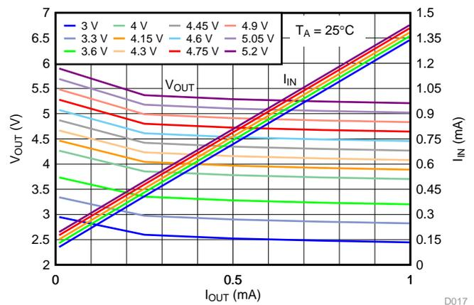
Figure 65. Output Voltage  $V_{OUT}$  and Input Current  $I_{IN}$  vs. Output Current  $I_{OUT}$  (0 to 1 mA) at  $25^{\circ}\text{C}$
