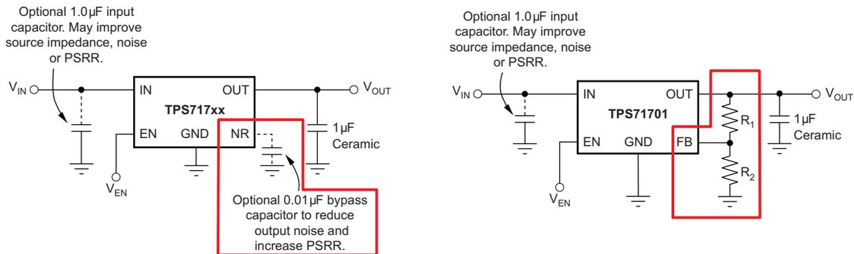
**Figure 31. TPS717xx — Typical Application Circuit: Fixed Output Voltage Version vs. Adjustable Output-Voltage Version**
