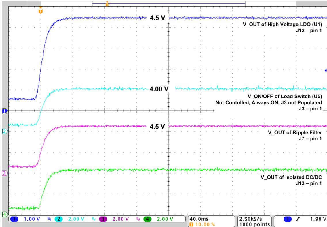
Figure 25. Load Switch Not Controlled but Always ON, 8-V Loop Input, Active-Current Limiter Used, R1 Active
