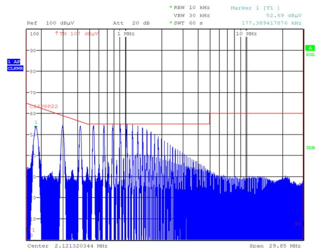
Conducted Noise on "N", 33V Loop Input, Scaled-Down Ripple Filter, Earthed Load
