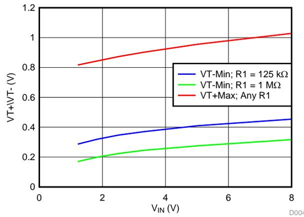
Figure 20. TPS27082L — ON/OFF Positive- and Negative-Going Threshold Voltage
