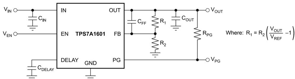
Figure 15. TPS7A1601 — Programming of Output Voltage and PG Delay Time
