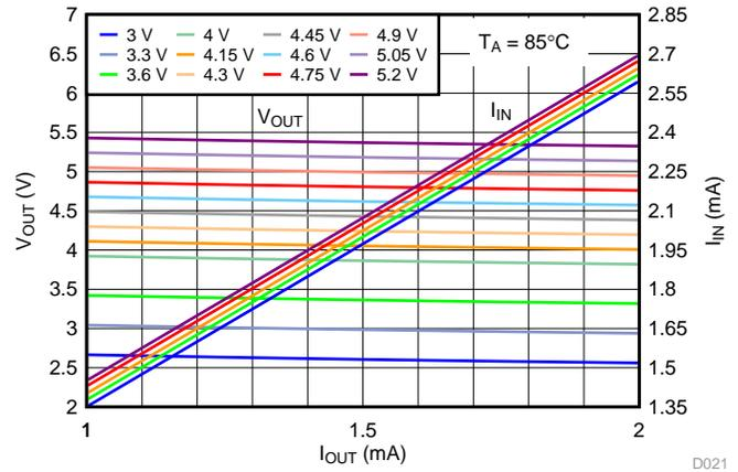
Figure 69. Output Voltage  $V_{OUT}$  and Input Current  $I_{IN}$  vs. Output Current  $I_{OUT}$  (1 to 2 mA) at 85°C
