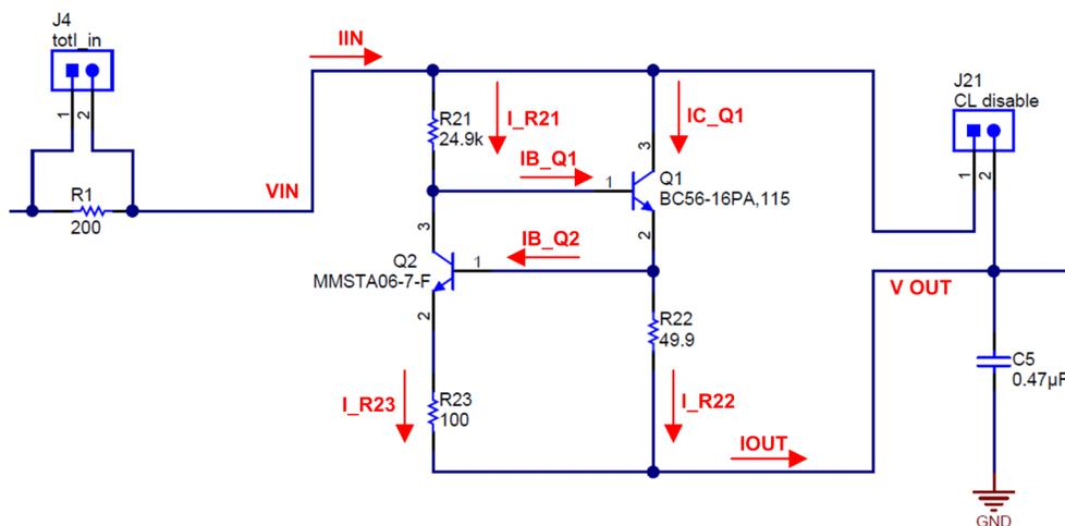
Figure 11. Active Current Limiter — Schematic and Operation
