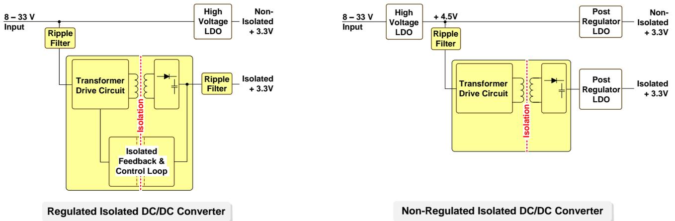
**Figure 39. Isolated DC/DC Converter: Regulated versus Nonregulated Control Approach**
