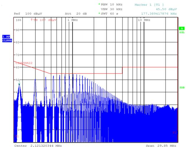
Conducted Noise on "L1", 33V Loop Input, Scaled-Down Ripple Filter, Earthed Load
