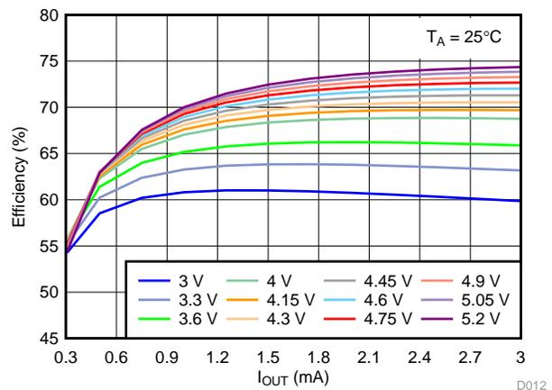
Figure 60. Efficiency vs. Output Current IOUT at  $25^{\circ}\text{C}$
