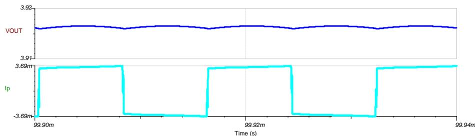
**Figure 53. Current in Primary Winding — 40  $\Omega$  (Simulation with TINA-TI)**
