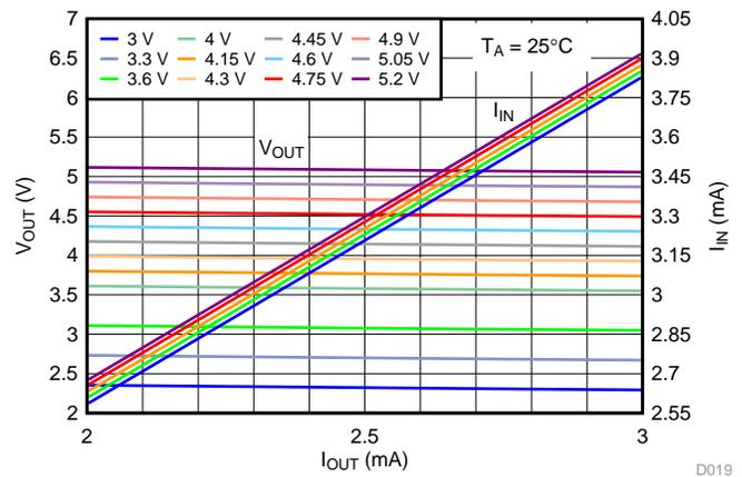
Figure 67. Output Voltage  $V_{OUT}$  and Input Current  $I_{IN}$  vs. Output Current  $I_{OUT}$  (2 to 3 mA) at  $25^{\circ}\text{C}$
