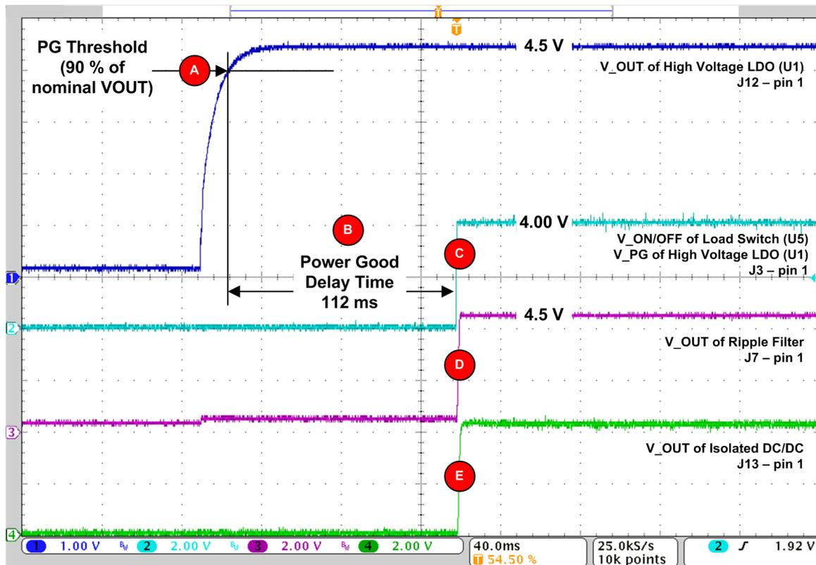
**Figure 22. Load Switch Controlled by Power Good, 33-V Loop Input, R1 Active**
