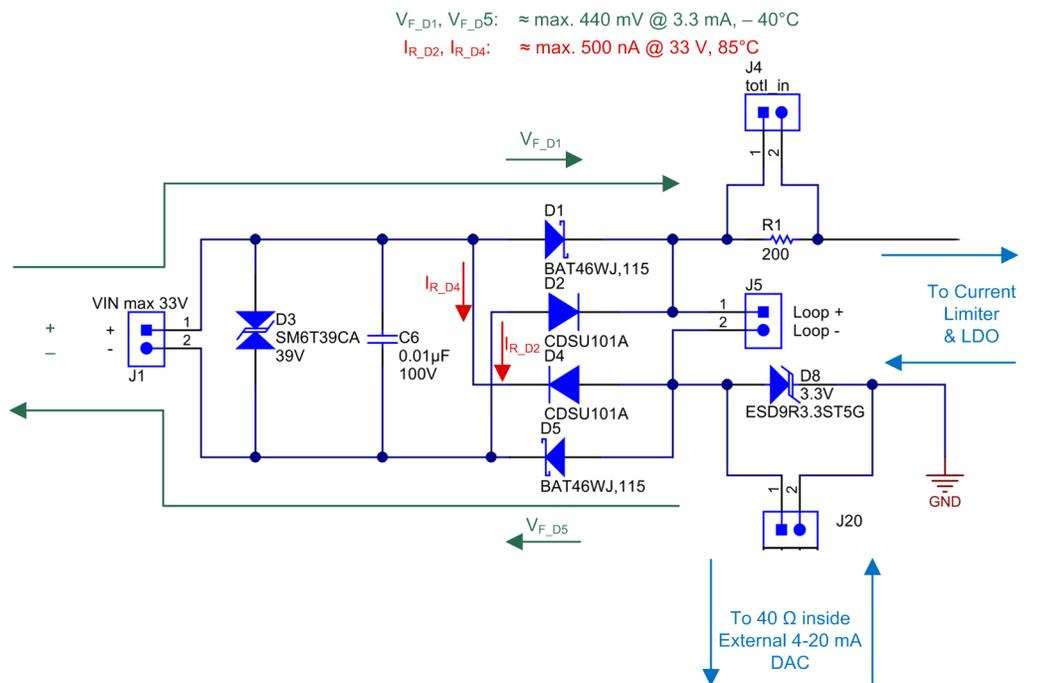
Figure 8. Input Reverse Protection — Loop Input with Correct Polarity
