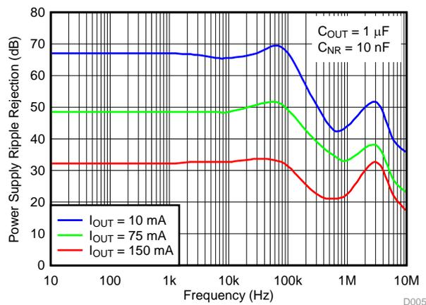
**Figure 30. TPS71733 — PSRR versus Frequency at V<sub>IN</sub> – V<sub>OUT</sub> = 0.25 V**
