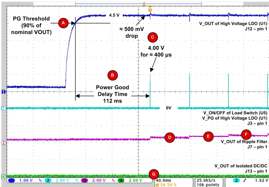
**Figure 23. Load Switch Controlled by Power Good, 8-V Loop Input, R1 Active**
