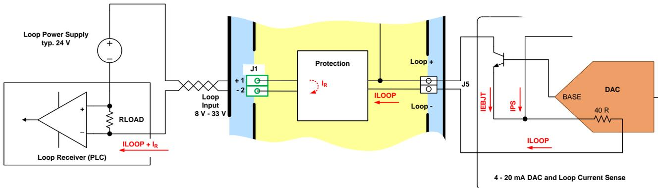
**Figure 5. Negative Impact of Leakage Current inside the Protection Block**
