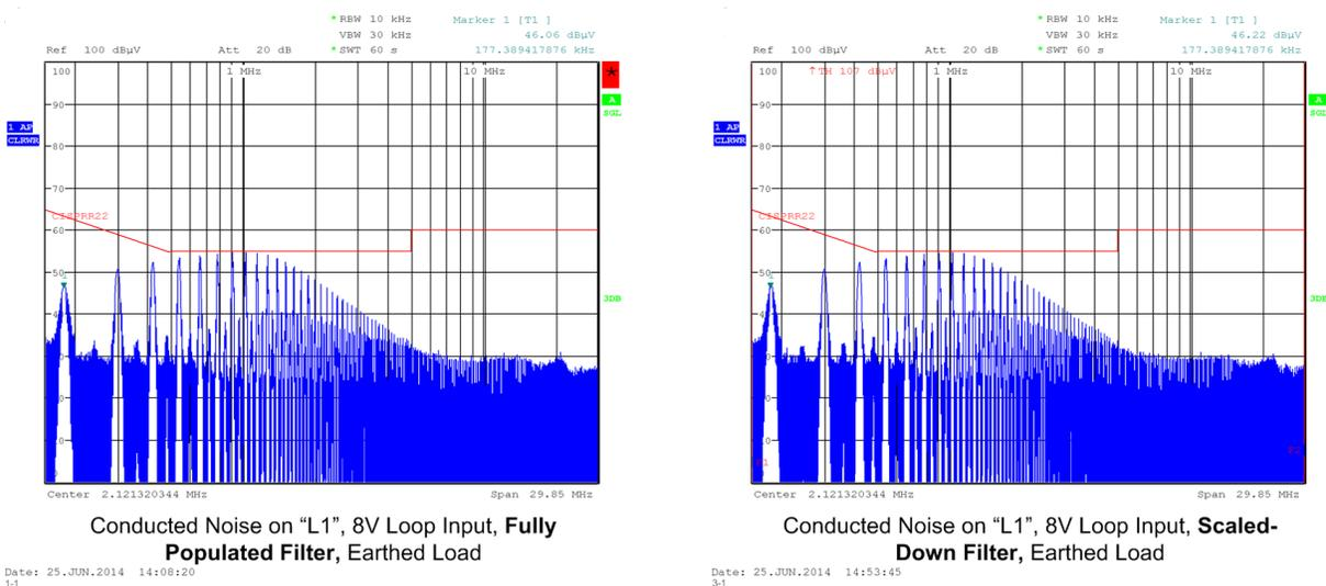
**Figure 28. Conducted Noise with 8-V Loop Voltage, Full Filter versus Scaled-Down Filter**
