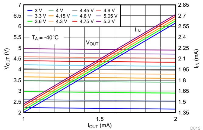
Figure 63. Output Voltage  $V_{OUT}$  and Input Current  $I_{IN}$  vs. Output Current  $I_{OUT}$  (1 to 2 mA) at  $-40^{\circ}\text{C}$
