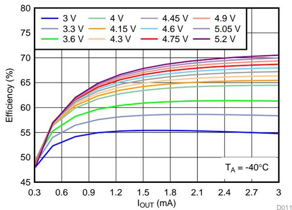
Figure 59. Efficiency vs. Output Current IOUT at  $-40^{\circ}\text{C}$
