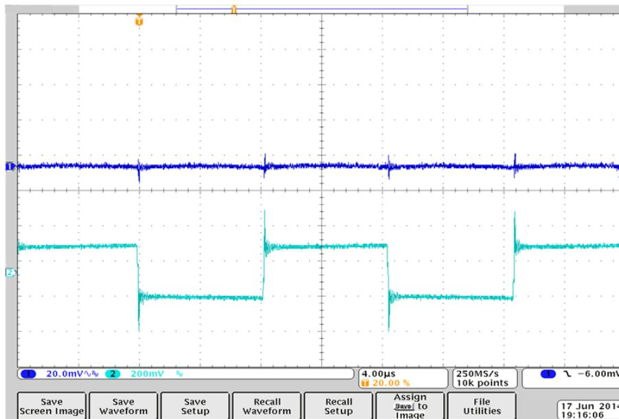
**Figure 52. Current in Primary Winding — 40  $\Omega$  (Real Measurement With Oscilloscope)**
