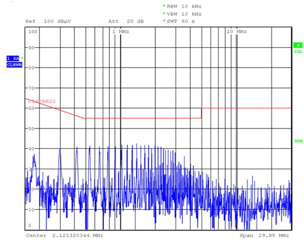
Conducted Noise on “L1”, 8V Loop Input, Full Ripple Filter, Non-Earthed Load
