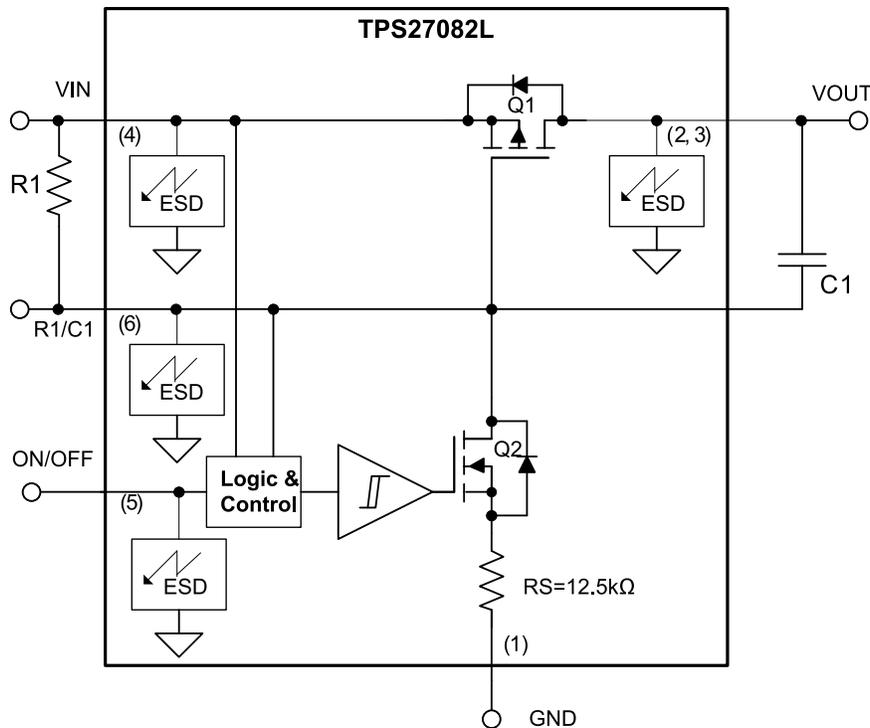
Figure 19. TPS27082L — Typical Application Diagram
