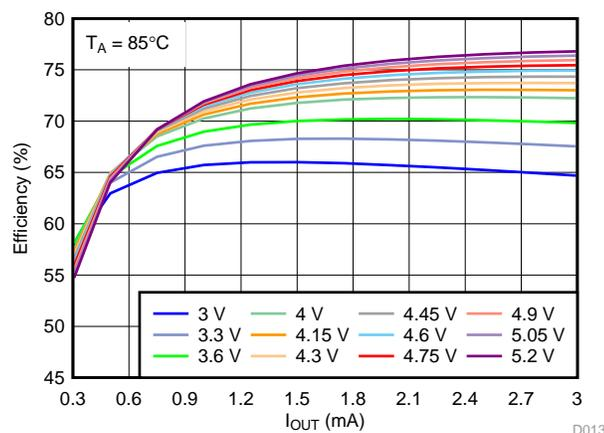
Figure 61. Efficiency vs. Output Current IOUT at  $85^{\circ}\text{C}$
