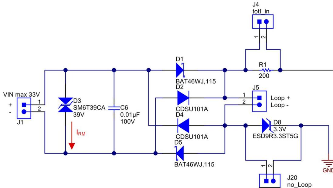
Figure 6. Input Overvoltage Protection
