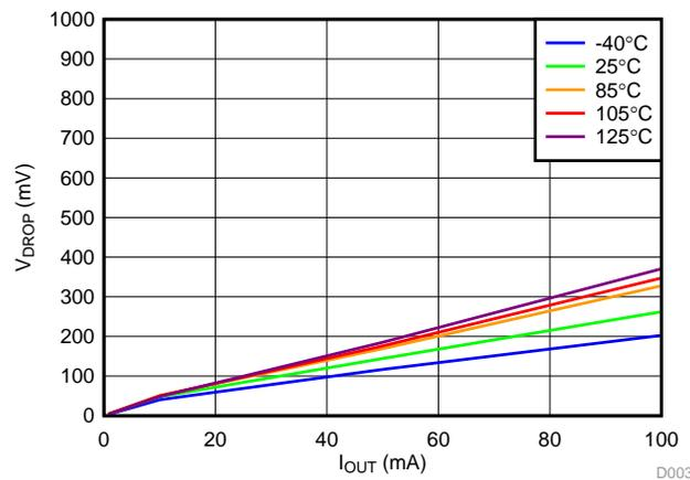
**Figure 16. TPS7A1601 - Dropout Voltage versus Output Current**
