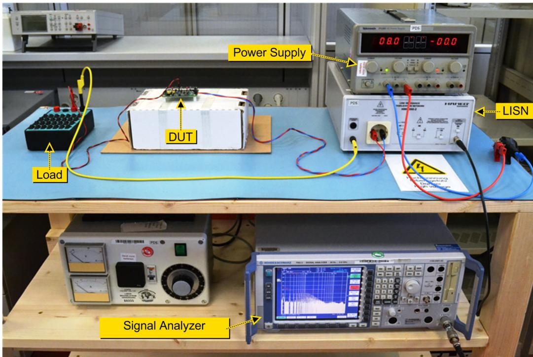
Figure 55. Pre-Compliance Conducted Noise Measurement — Test Setup
