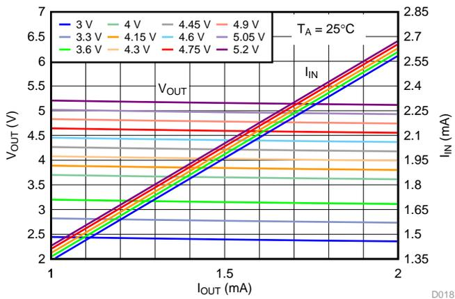
Figure 66. Output Voltage  $V_{OUT}$  and Input Current  $I_{IN}$  vs. Output Current  $I_{OUT}$  (1 to 2 mA) at  $25^{\circ}\text{C}$
