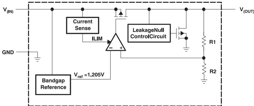
Figure 34. TPS71533 — Functional Block Diagram
