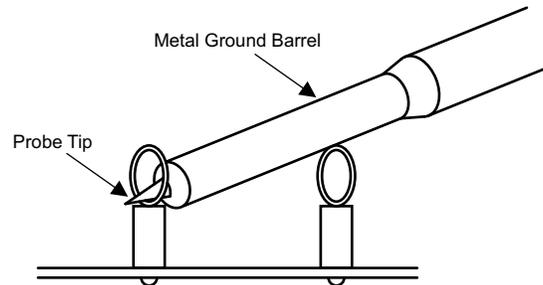
**Figure 51. Tip and Barrel Method for Noise-Free Measurement**
