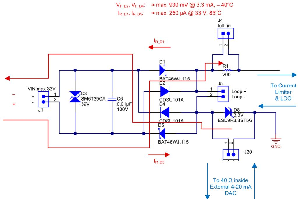
**Figure 9. Input Reverse Protection — Loop Input with Reverse Polarity**
