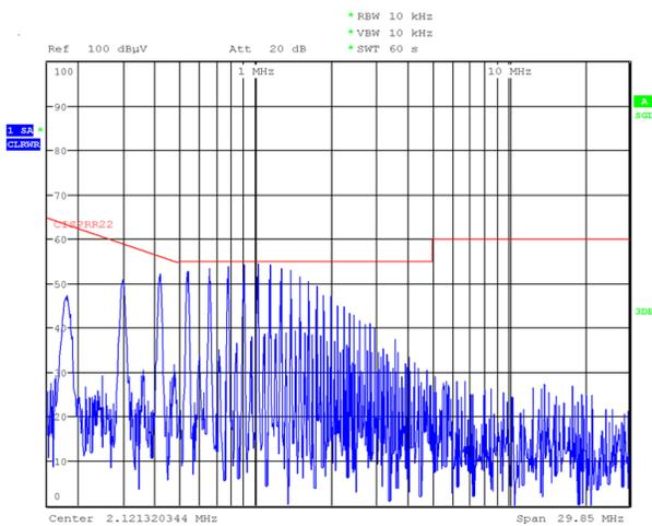
Conducted Noise on “L1”, 8V Loop Input, Full Ripple Filter, Earthed Load
