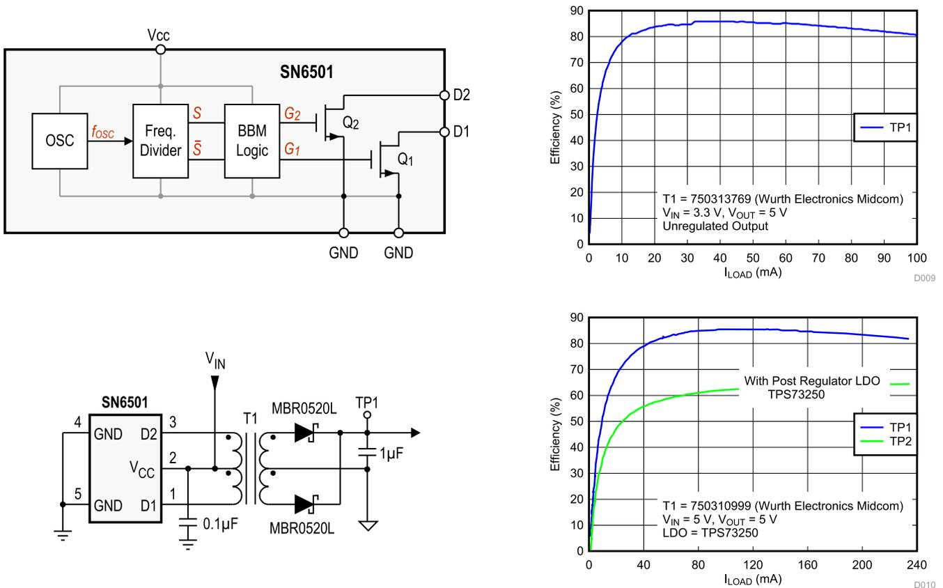
Figure 42. SN6501 — Block Diagram, Schematic, and Efficiency
