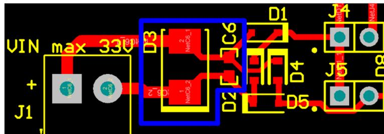
Figure 7. Input Overvoltage Protection — Layout Details
