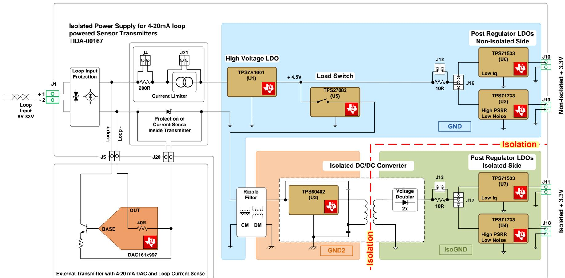
Figure 3. TIDA-00167 Block Diagram
