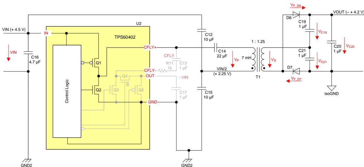
Figure 48. Simplified Schematic of Isolated DC/DC Converter
