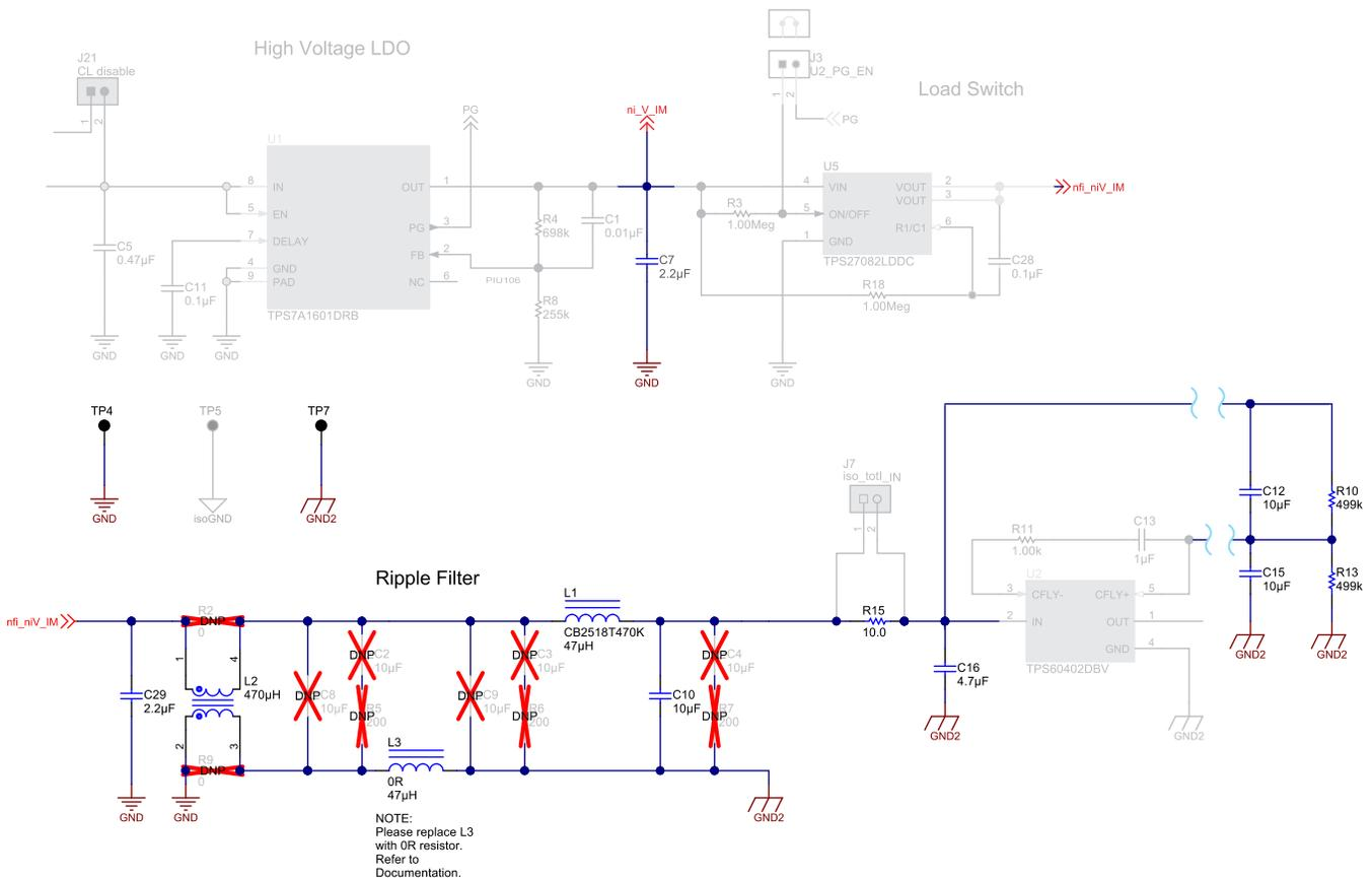
Figure 26. Ripple Filter — Circuit Implementation
