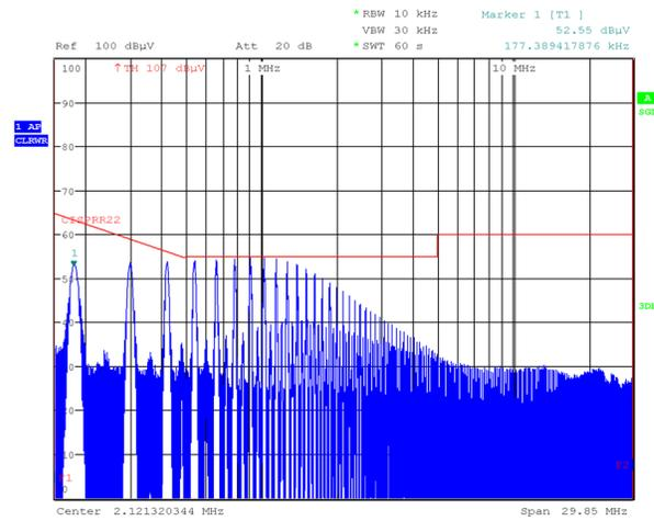
Conducted Noise on "N", 8V Loop Input, Scaled-Down Ripple Filter, Earthed Load
