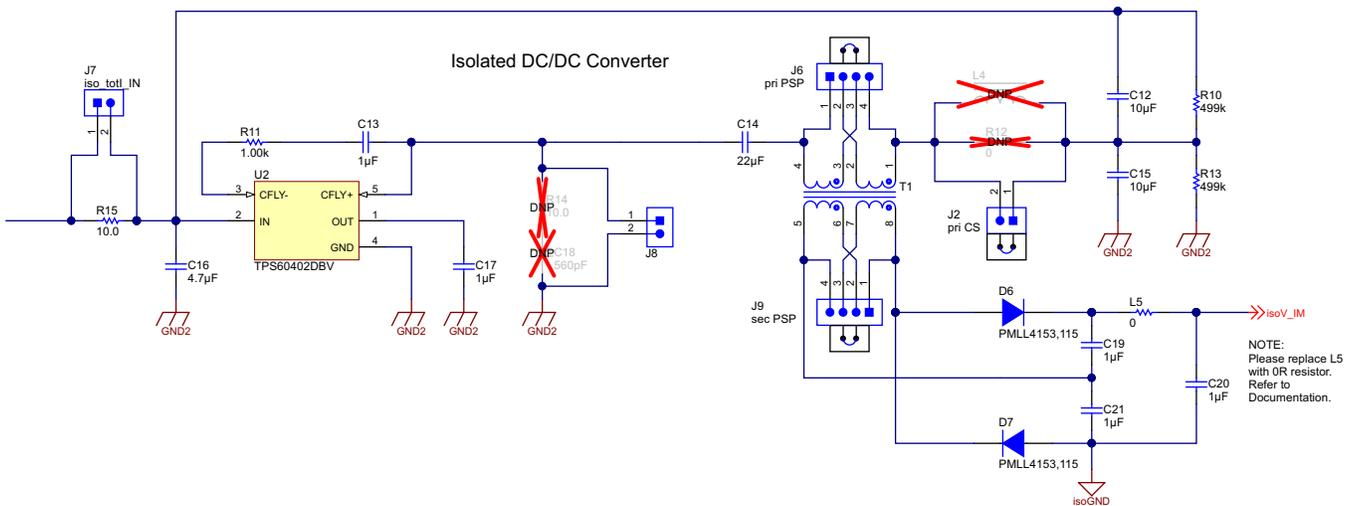
**Figure 50. Isolated DC/DC — Real Implementation**
