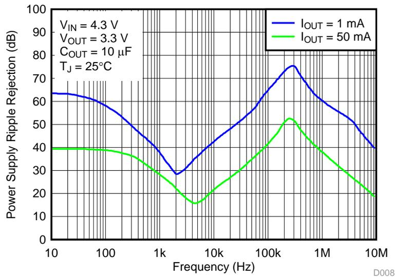
**Figure 35. TPS71533 — PSRR versus Frequency at  $V_{IN} - V_{OUT} = 1\text{ V}$**
