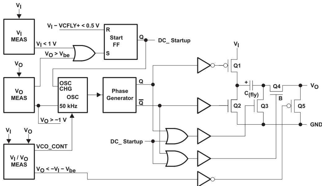
**Figure 46. TPS60400 Family — Functional Block Diagram**
