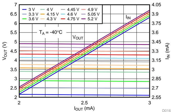
Figure 64. Output Voltage  $V_{OUT}$  and Input Current  $I_{IN}$  vs. Output Current  $I_{OUT}$  (2 to 3 mA) at  $-40^{\circ}\text{C}$
