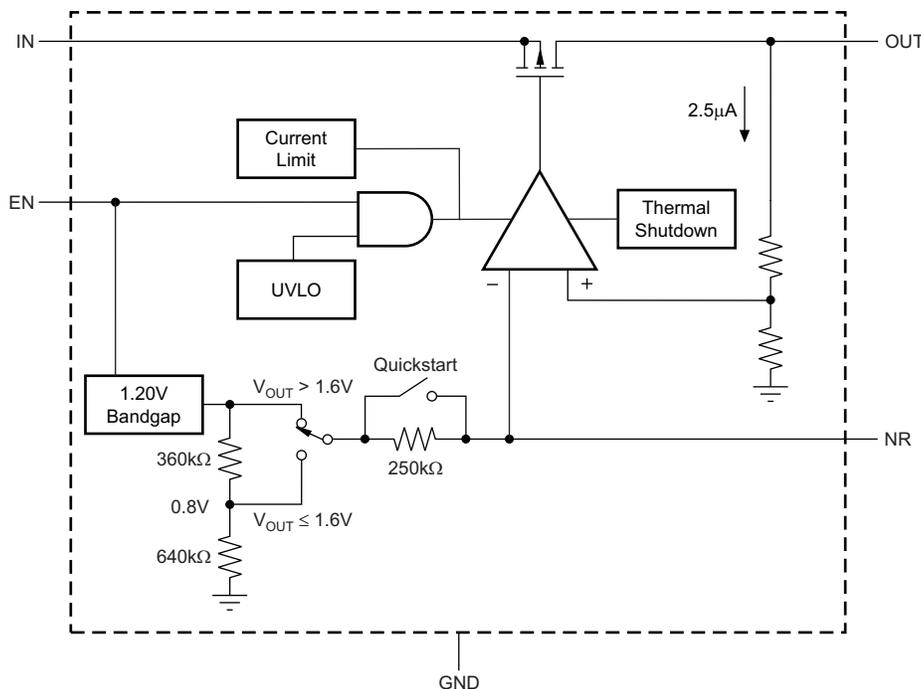
**Figure 32. TPS71733 — Functional Block Diagram**
