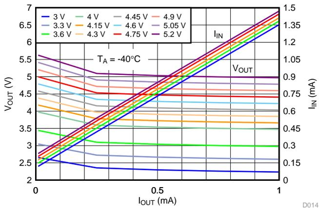
Figure 62. Output Voltage  $V_{OUT}$  and Input Current  $I_{IN}$  vs. Output Current  $I_{OUT}$  (0 to 1 mA) at  $-40^{\circ}\text{C}$
