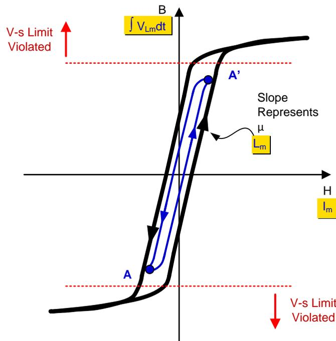
**Figure 44. Hysteresis Curve of Ferrite and of Specific Inductor**
