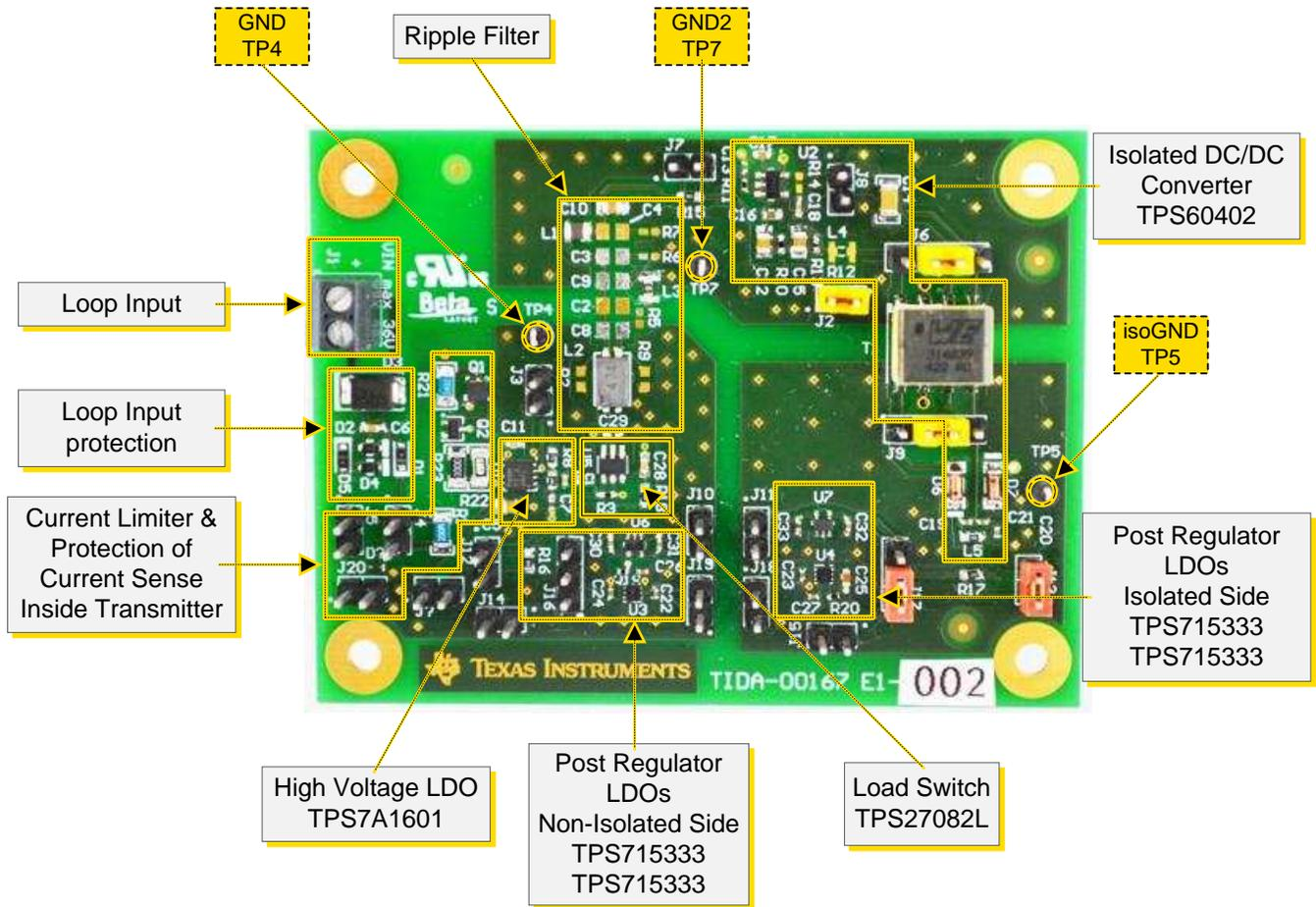
**Figure 4. TIDA-00167 PCB Assembly View**
