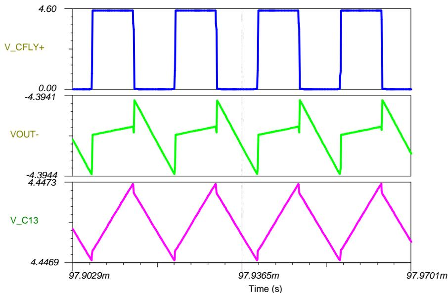
**Figure 49. Charge Pump Operation**
