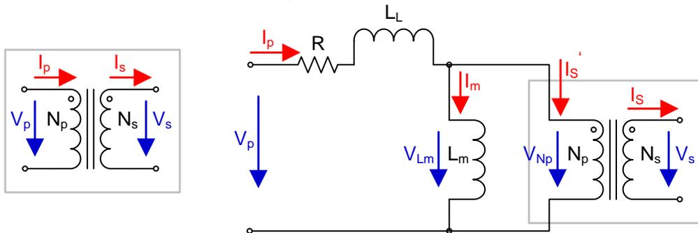
Figure 43. Ideal Transformer versus Simplified Model of Real Transformer
