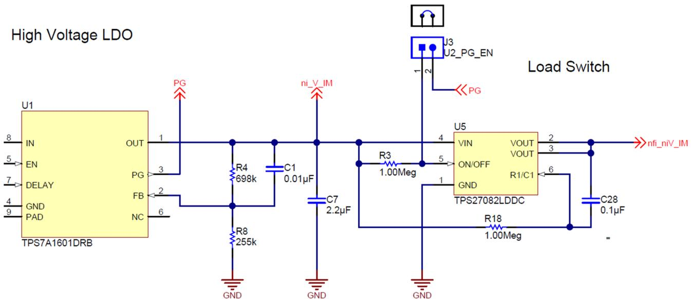
Figure 21. Load Switch — Circuit Implementation
