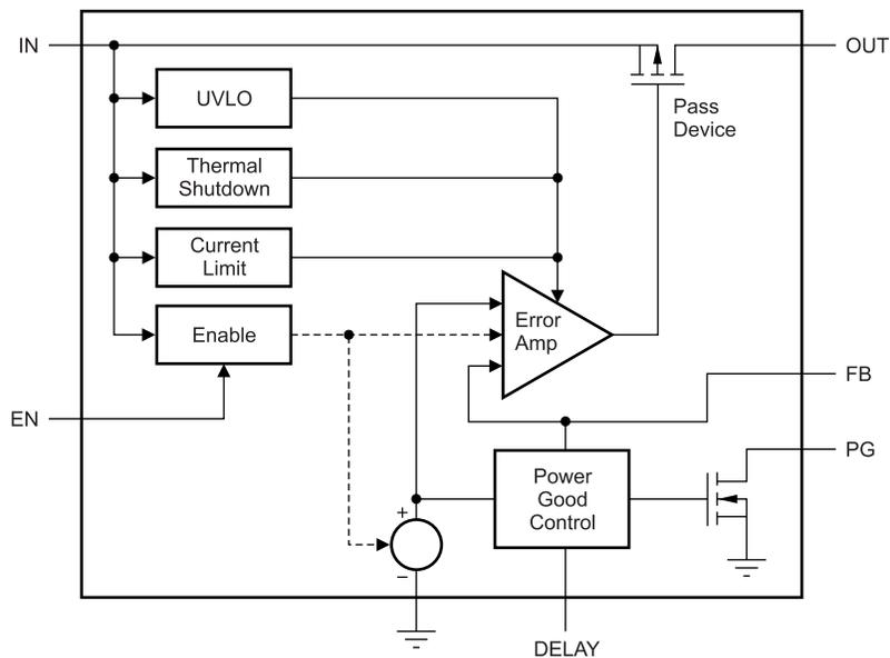
Figure 14. TPS7A1601 Block Diagram
