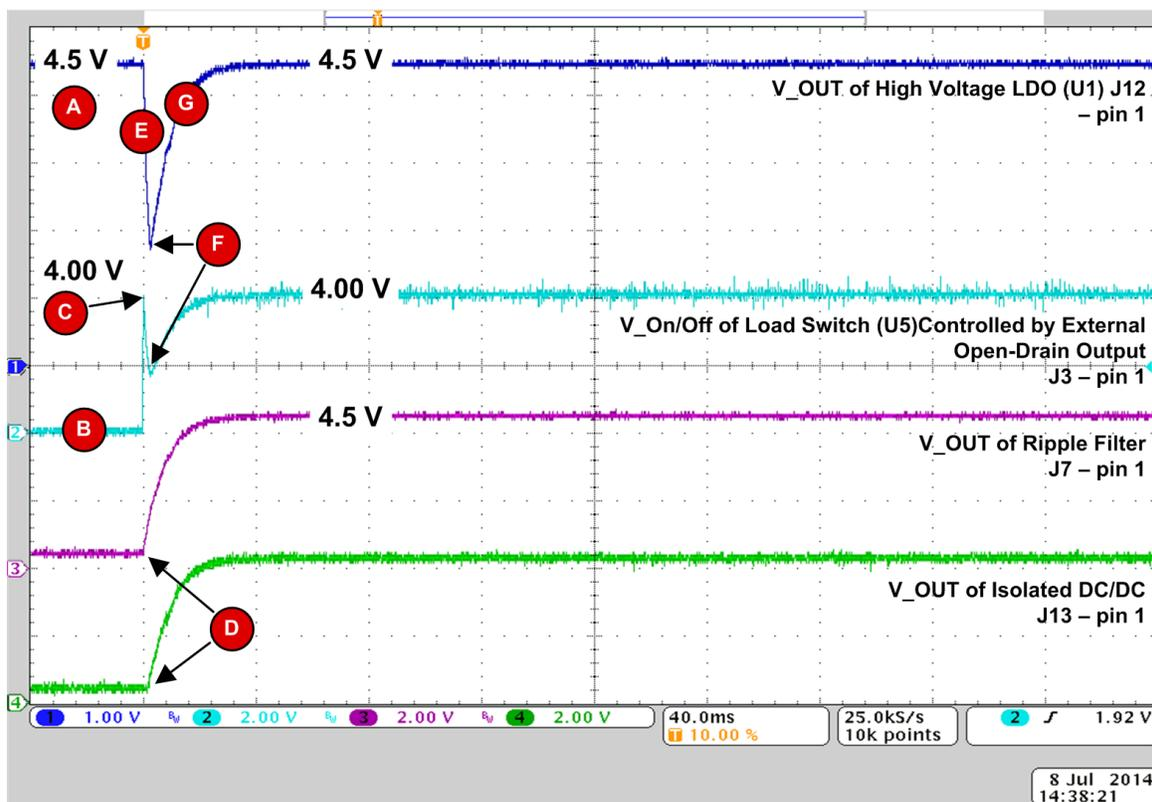
Figure 24. Load Switch Controlled by External ENABLE Signal, 8-V Loop Input, Active Current Limiter Used and R1 Active
