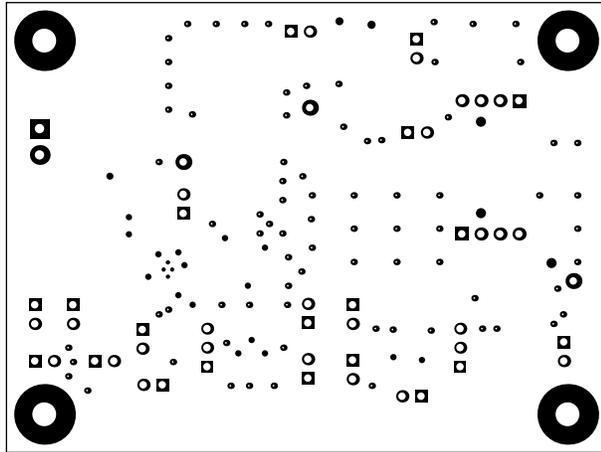
**Figure 76. Bottom Solder Mask**
