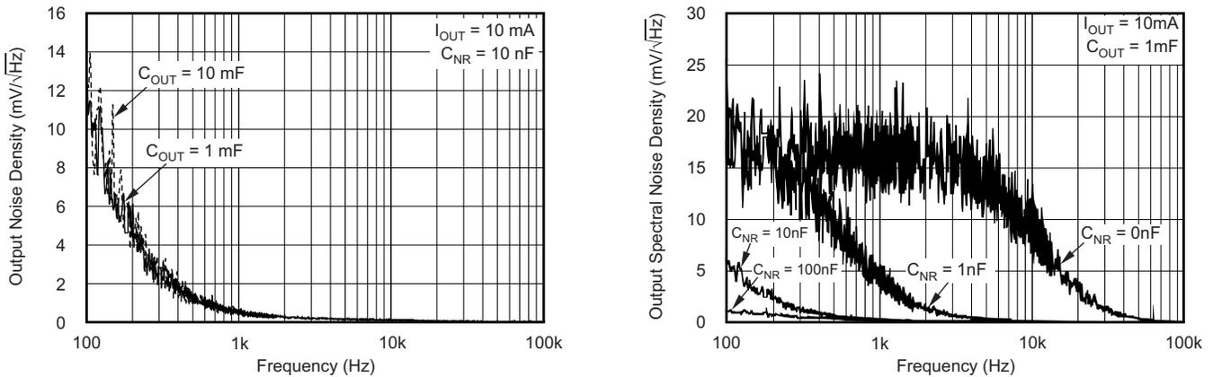
Figure 33. TPS71733 — Effect of Noise Reduction and Output Capacitor on Output-Noise Density
