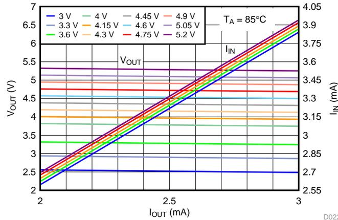
Figure 70. Output Voltage  $V_{OUT}$  and Input Current  $I_{IN}$  vs. Output Current  $I_{OUT}$  (2 to 3 mA) at 85°C
