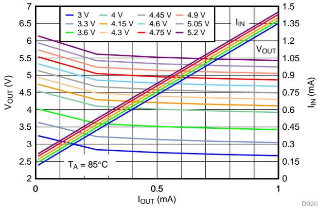
Figure 68. Output Voltage  $V_{OUT}$  and Input Current  $I_{IN}$  vs. Output Current  $I_{OUT}$  (0 to 1 mA) at 85°C
