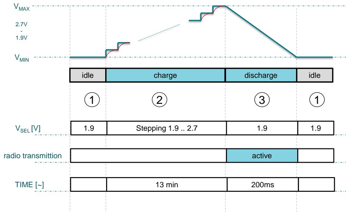
Figure 3: Recharge Cycle Sequencing
