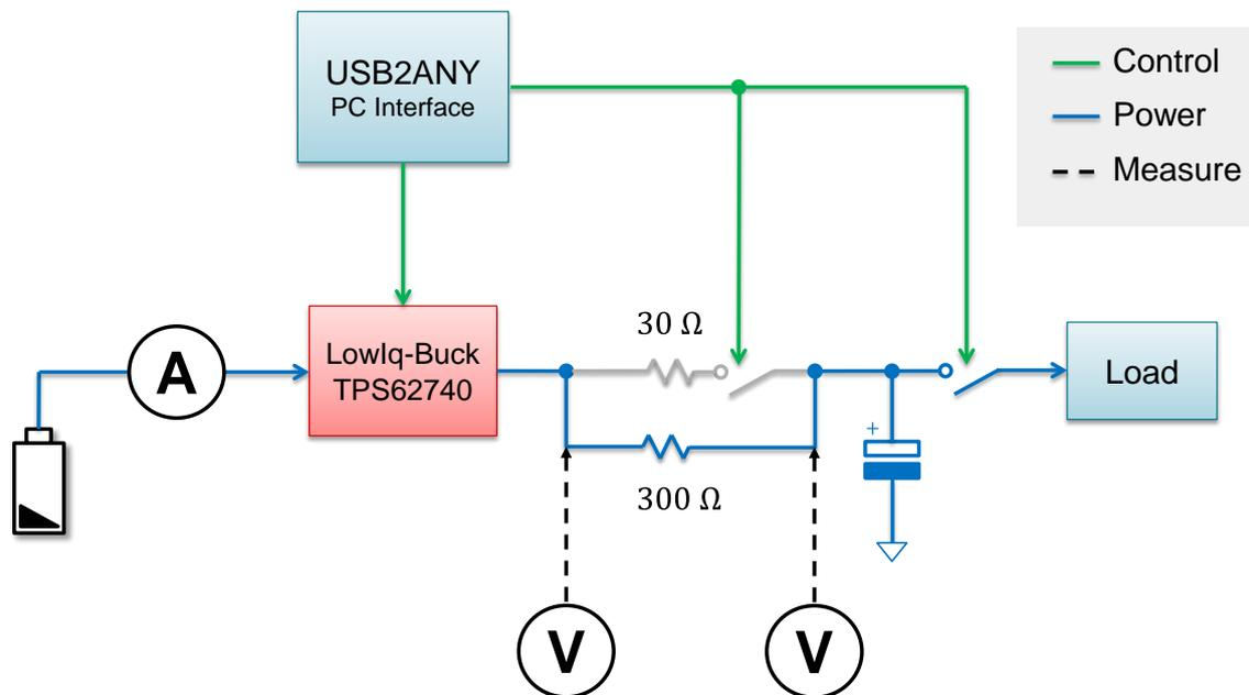
Figure 6: Start-up circuit configuration
