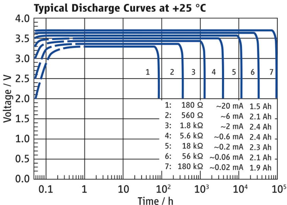
Figure 1: typ. discharge curve of a TADIRAN SL-360 over several loads <sup>1</sup>
