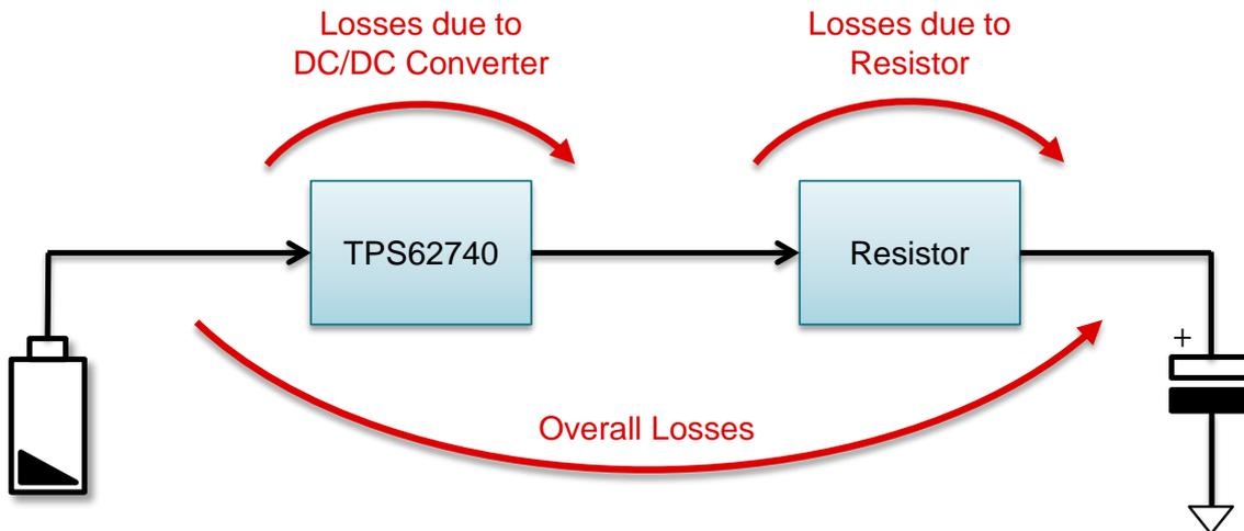
Figure 10: Conversion efficiency
