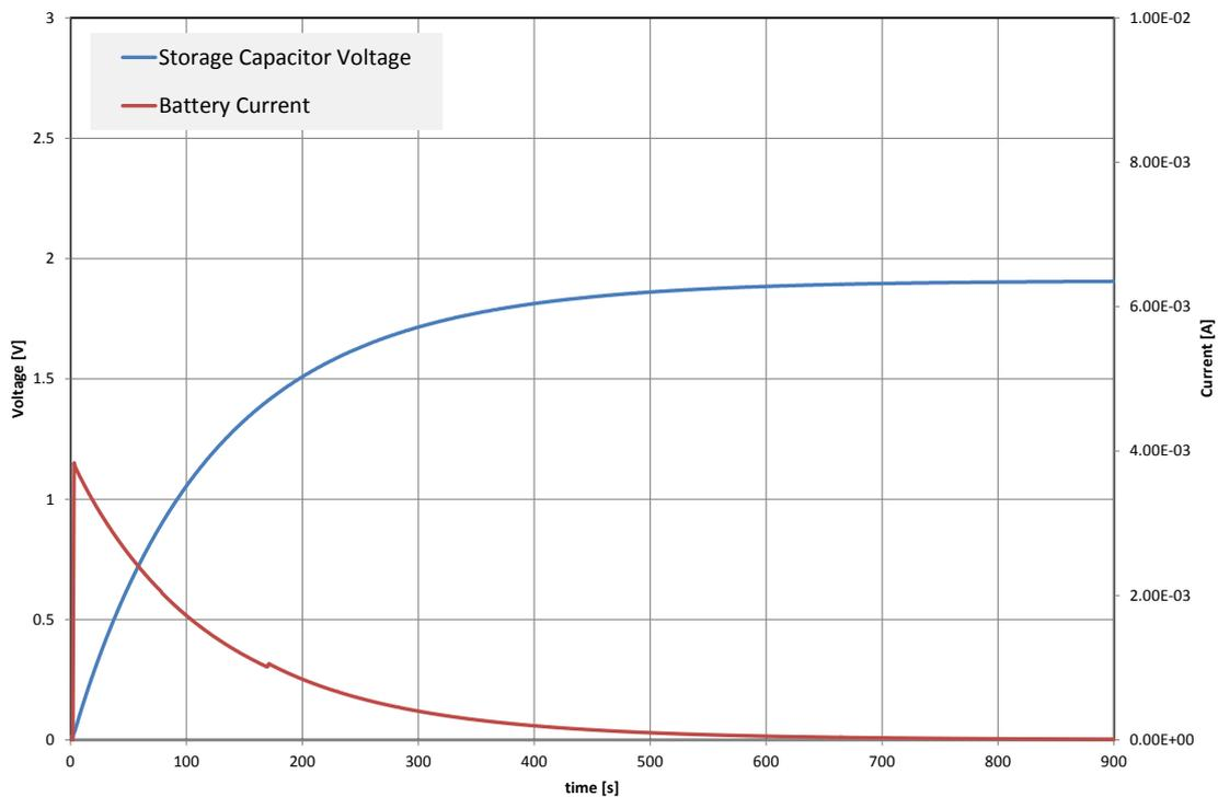
Figure 7: Battery current and capacitor voltage during pre-charge
