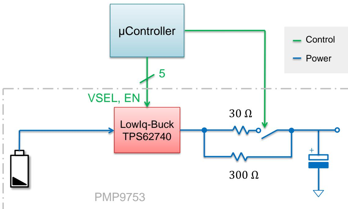
Figure 4: Reference design block diagram
