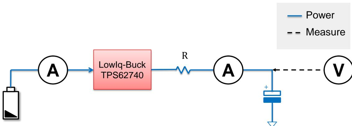
Figure 12: Energy conversion efficiency measurement setup
