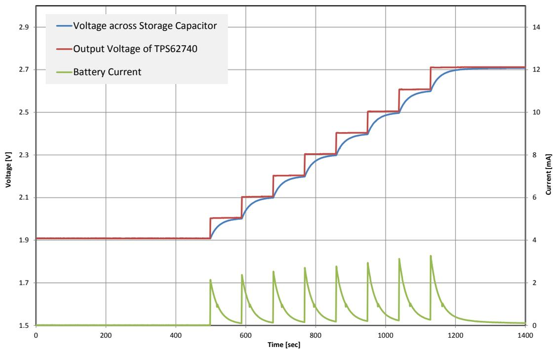
Figure 9: Charging waveforms
