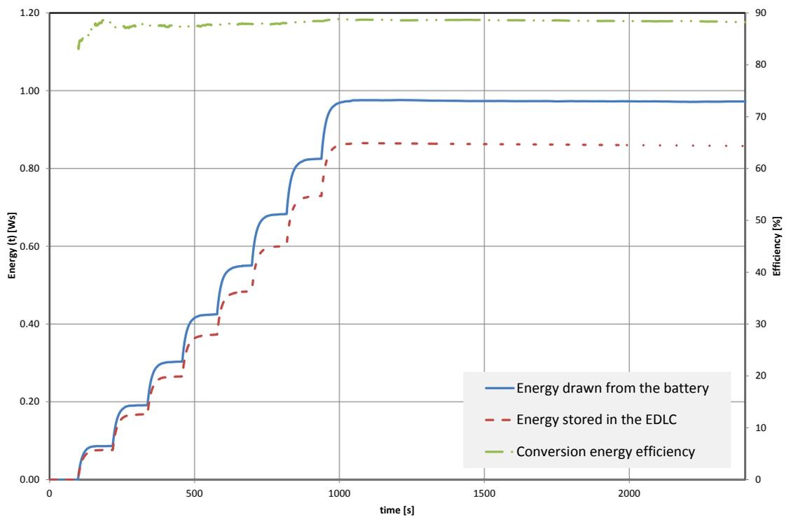
Figure 14: Energy conversion efficiency
