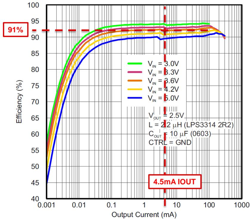
Figure 11:TPS62740: Efficiency vs. output current
