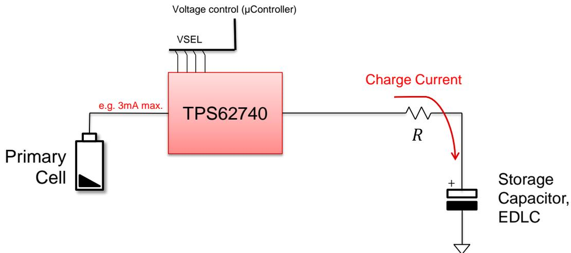
**Figure 2: Simplified charging block diagram**
