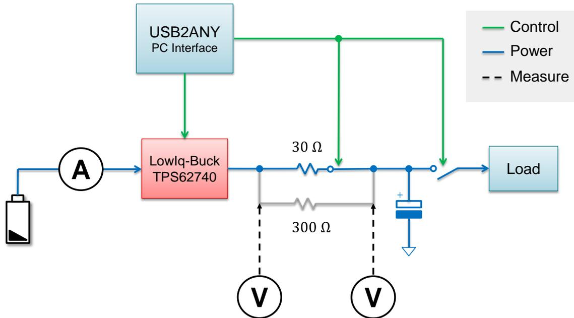
Figure 8: Diagram of the measurement setup
