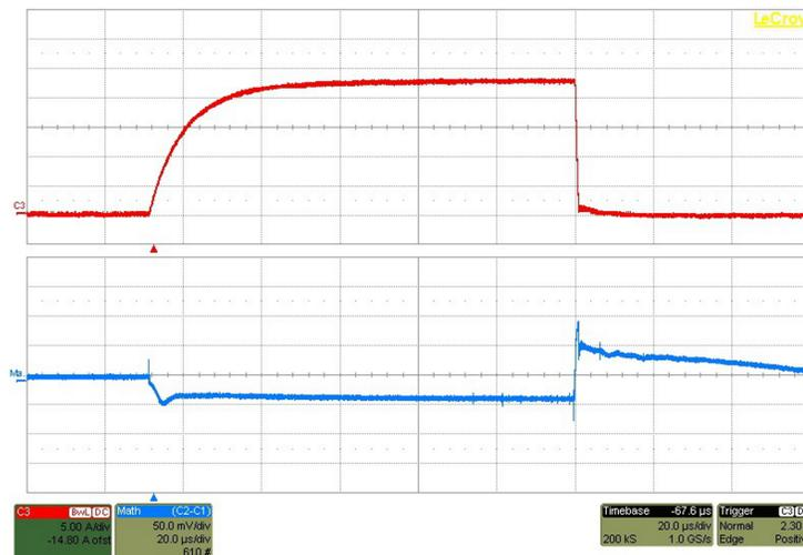
Figure 38. Load Transient 23 A
