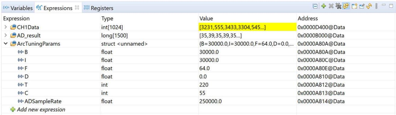
**Figure 3-5. Expressions Window for 20 kHz Sinusoidal Input Current**
