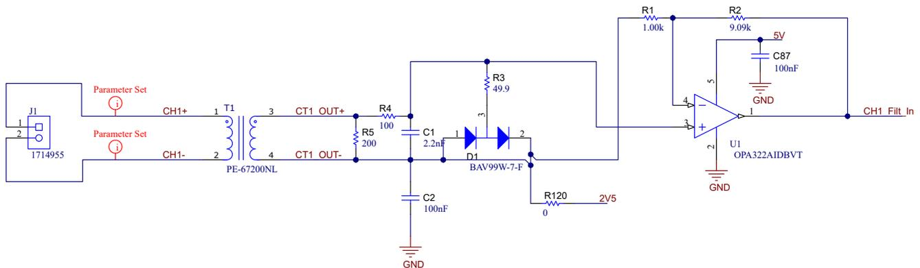
Figure 2-2. Schematic Current Transformer Circuit and Gain Stage
