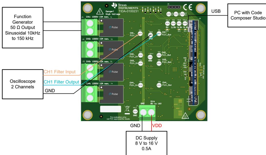
**Figure 3-1. Hardware and Software Validation Setup**
