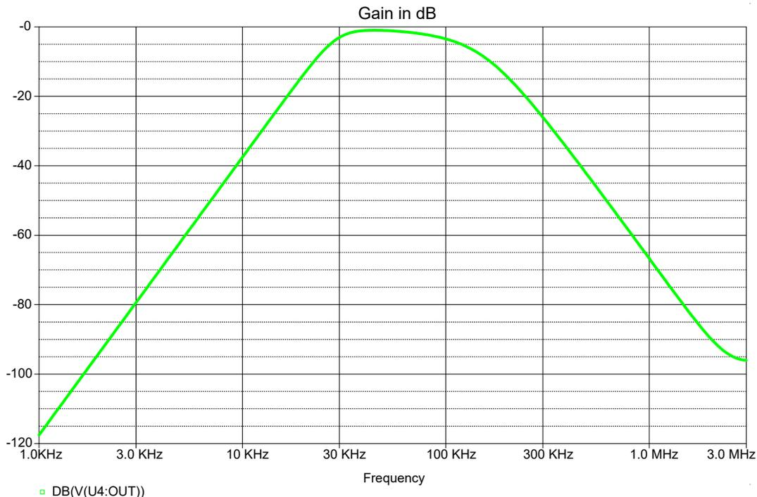
**Figure 2-4. Simulated Magnitude of the Frequency Response of the Filter Stage**
