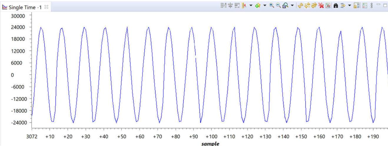
**Figure 3-6. Graph of CH1Data at 20-kHz Sinusoidal Input Current**
