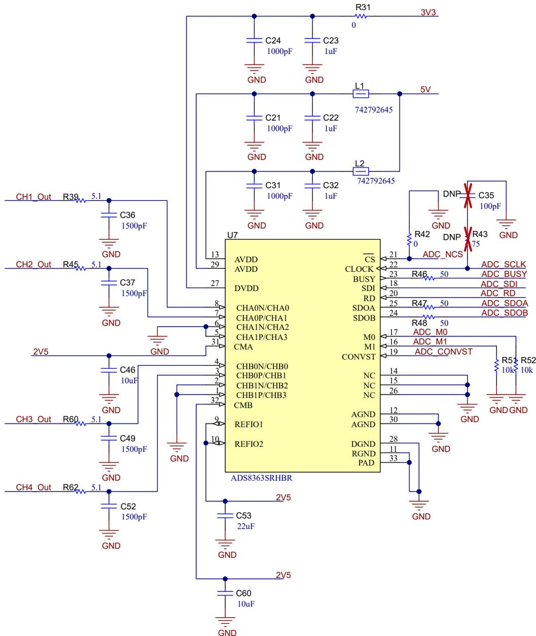
Figure 2-5. Schematic Analog-to-Digital Conversion With ADS8363
