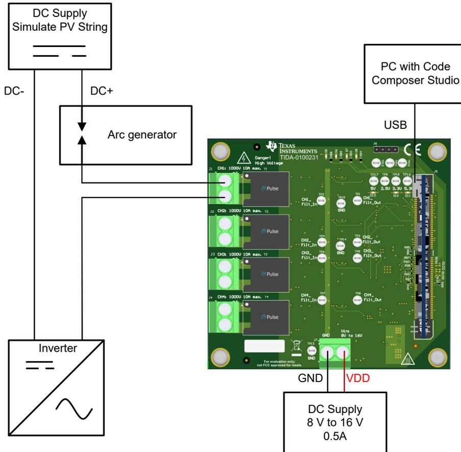
**Figure 3-2. Arc Detection Test Setup**
